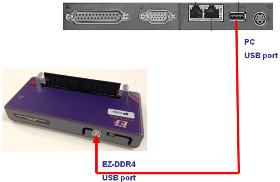
Figure 4-0 : EZ -SPD DDR4 PC Interface Control Setup.
