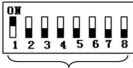
The figure shows: Address of the dome device: No. 1
