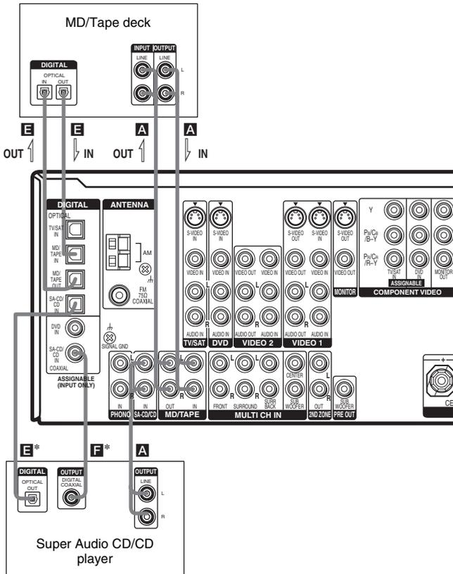
\* Connect to either the SA-CD/CD COAXIAL IN or the SA-CD/CD OPTICAL IN jack. We recommend making connections to the SA-CD/CD COAXIAL IN jack.
