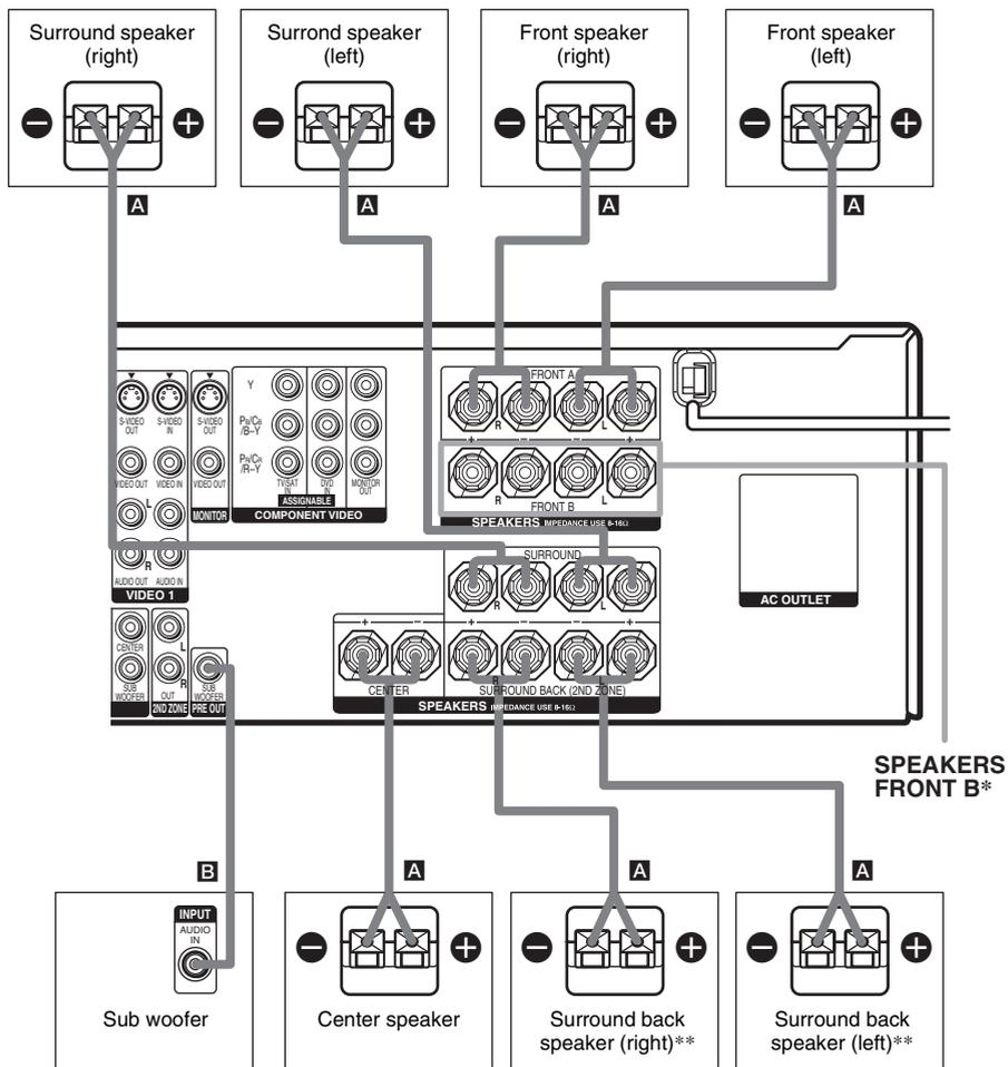
\* If you have an additional front speaker system, connect them to the SPEAKERS FRONT B terminals. You can select the front speakers you want to use with SPEAKERS (OFF/A/B/A+B) button. For details, see “Selecting the speaker system” (page 42).
