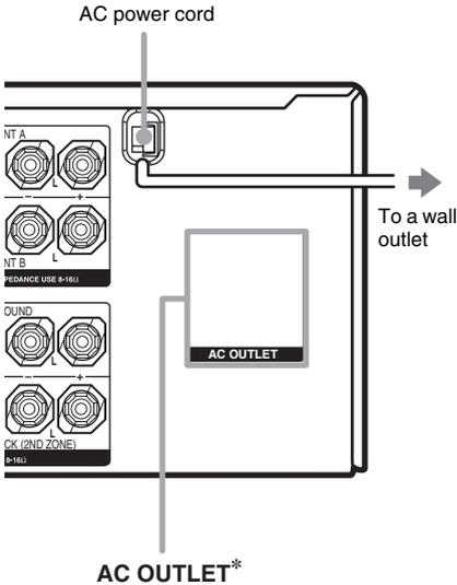
\* The configuration, shape, and number of AC outlets vary according to the area code.
