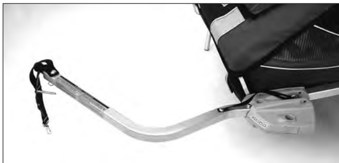
Correctly installed hitcharm.
