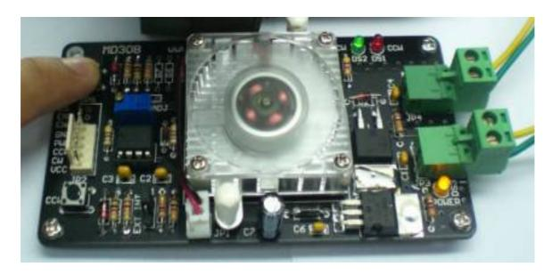
c. If CCW button is press, motor will run counter clockwise and CCW indicator LED (red) will turn ON.
