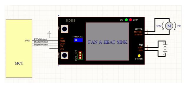
As for PWM pin in External PWM mode, user may provide a constant 5V or 12V to it if speed control is not required.
