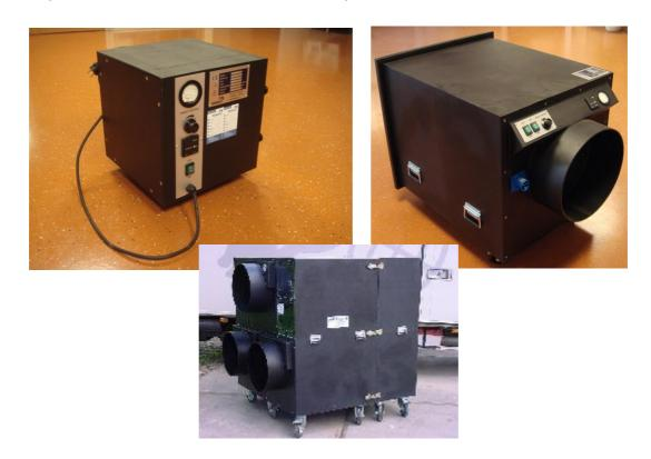
The required capacity of the device depends on the volume of the workspace and the number of leaks in the sheathing. When creating negative pressure at least 6 to 8 air changes per hour have to be assumed and a pressure of 30-40 Pascal.
