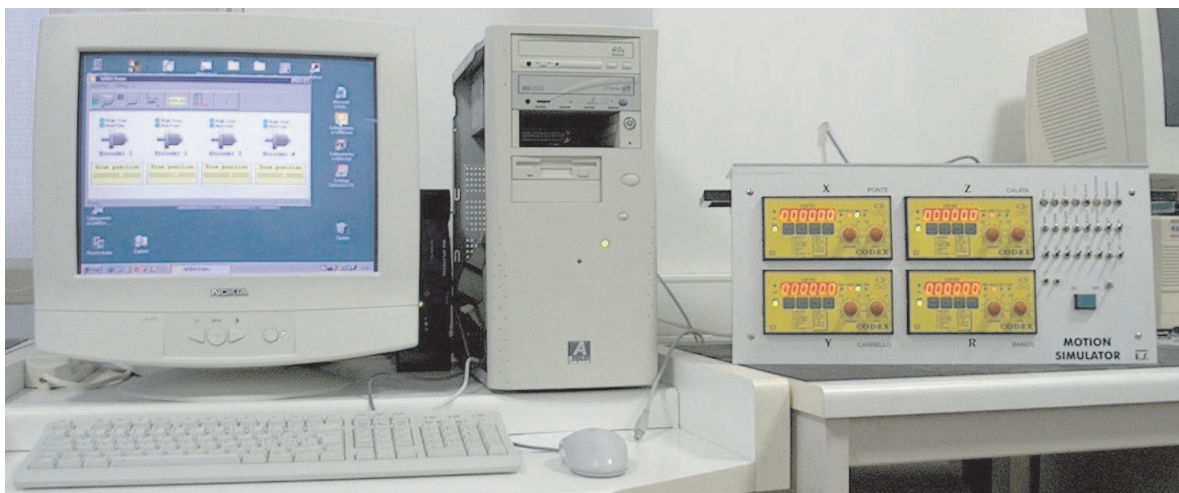
A 4-ENCODER-SIMULATOR BOX USED TO TEST THE BOARD PC864
