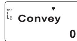
**3. Press the [▼] key repeatedly until the desired tag name number is called up.****4. Press the [SET] key.**
