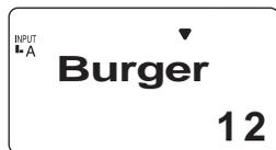
3. Press the [▼] key repeatedly until the tag to be confirmed is displayed on the screen.
