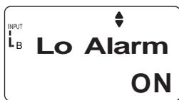
9. Use either the [▼] or [▲] key to set the lower-limit temperature alarm function ON/OFF.
