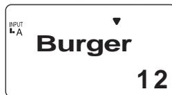
3. Press the [▼] key repeatedly until the tag to be modified is displayed on the screen.
