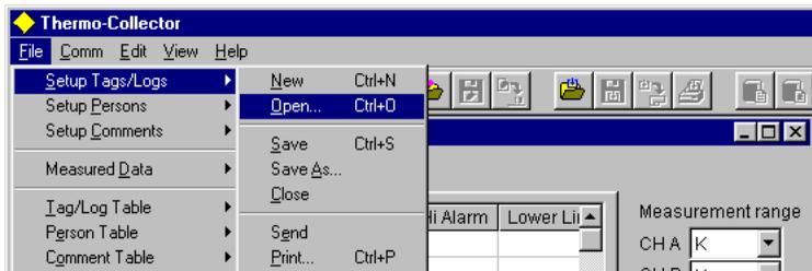
1. Select "Open" in the "Setup Tags/Logs" menu accessed from the "File" menu. The "Open" window is displayed.
