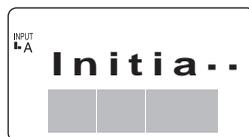
In two minutes, all the data set in the main unit is erased and the “Initial” screen is restored. Press the [ESC] key repeatedly to return to the Home screen.
