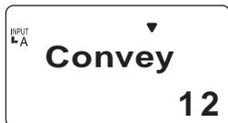
3. Press the [▼] key repeatedly until the log to be deleted is displayed on the screen.
