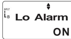
7. Use either the [▼] or [▲] key to select ON/OFF of the lower-limit temperature alarm function.
