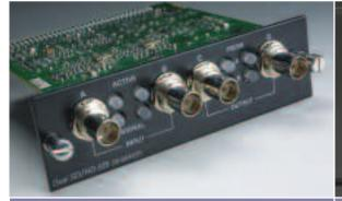
The Dual SD/HD-SDI Input Module is an optional module that allows for the connection of both a Standard Definition and a High Definition Serial Digital Input, each with their own loop-through.
