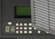
Direct key access to the most-used major functions and auto set-up for automatic set-up of sources with correct brightness, contrast and position – means operation and set-up of the Christie Roadster Series are intuitive.
