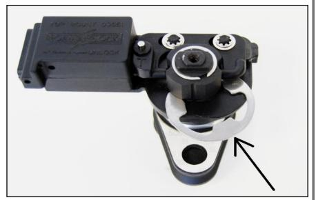
5) Reinstall the Emergency Handle and cables to the rotary latch, route the passenger side cable through the cable guide hole on the Lock Module the out to the rotary latch.
