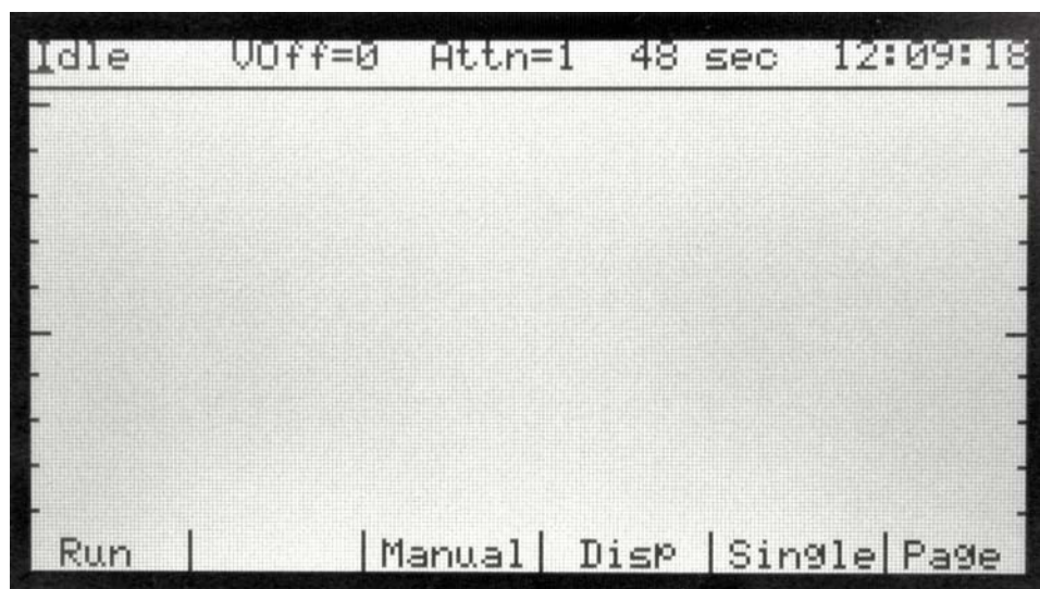
Figure 26. Run / Chromatogram screen in the Idle state, and the mode displayed upon initial power up
