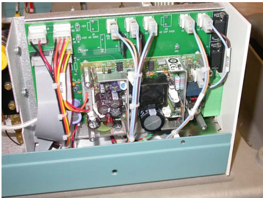
Figure 86. Main DC Power Supply with Shield Removed
