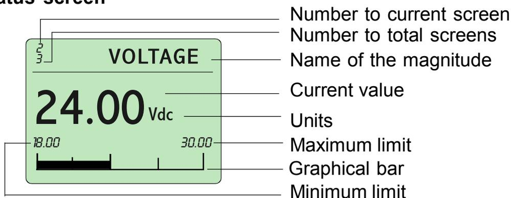
The status screens show the actual values of the magnitudes that the equipment controls. In the normal working mode, the equipment shows the status screen that the user has chosen like preferring magnitude of visualization. In order to move around among the different status screens of status, press ▲▼.
