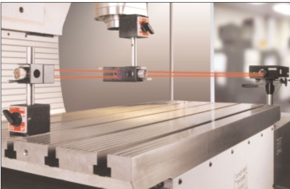
X axis linear positioning measurement on a VMC
