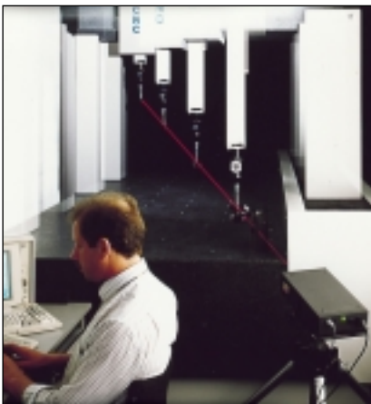
CMM space-diagonal calibration using laser measurement system.
