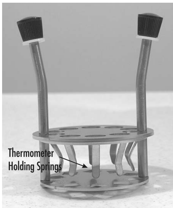
Figure 6 Thermometer Holding Carousel
