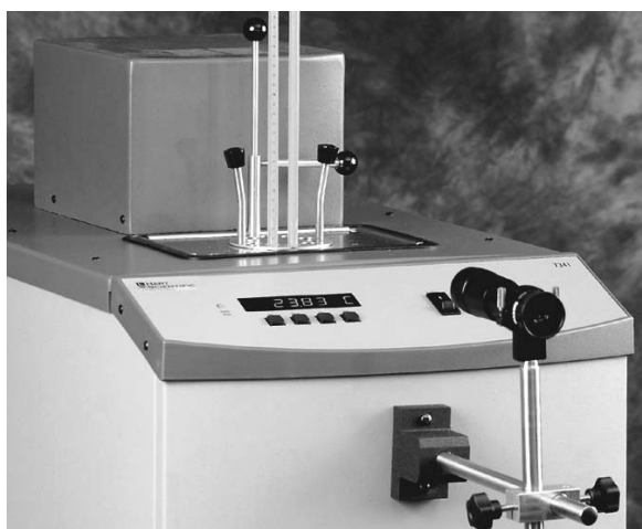
Figure 5 2019 Assembly in Place with Optional Magnifying Scope
