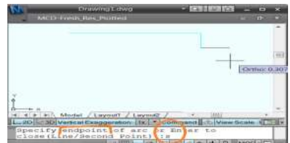
S9 – Type S to select option of picking second point of the arc
