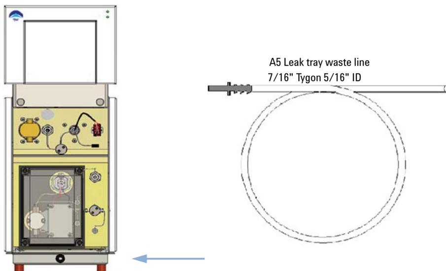
**Figure 17** Leak Tray Waste Line
