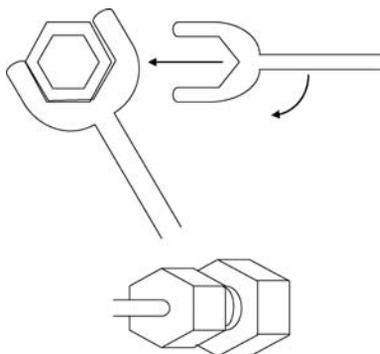
**Figure 4** Proper tightening of Fittings
