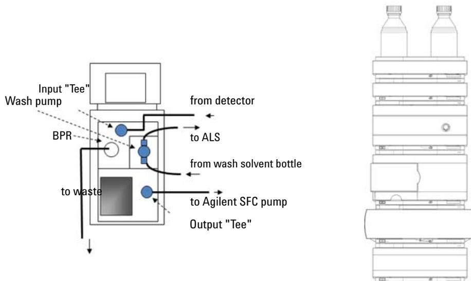
Figure 2 Agilent 1260 Infinity Analytical SFC System
