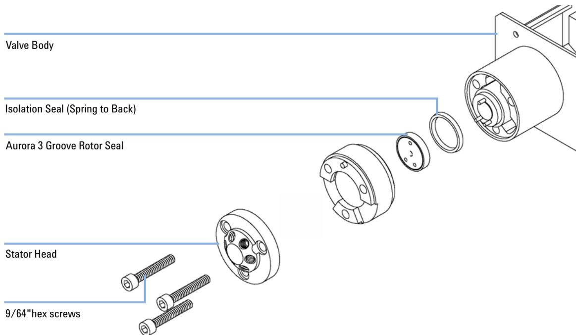
**Figure 21** Exploded View of the Autosampler Injection Valve
