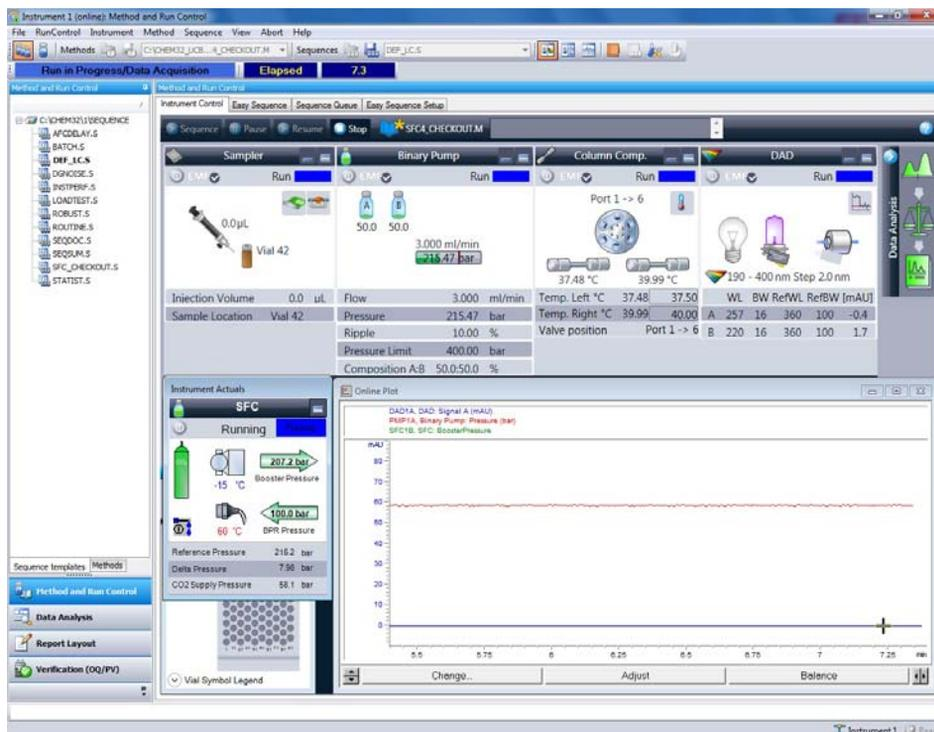
When the wash pump icon is clicked, the wash pump starts pumping for 30 seconds and flushes the autosampler metering, loop, needle and needle seat with solvent. Typically, modifier solvent is used to flush the autosampler. The wash pump is controlled by the Agilent SFC autosampler via the built-in BCD board, and works independently of the current state of the Aurora Fusion A5.
