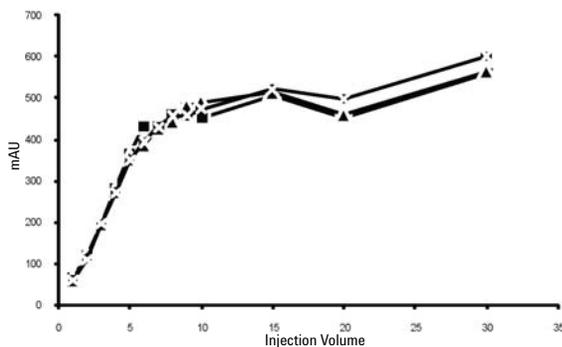
**Figure 27** Plot showing loss of efficiency with large injection volume
