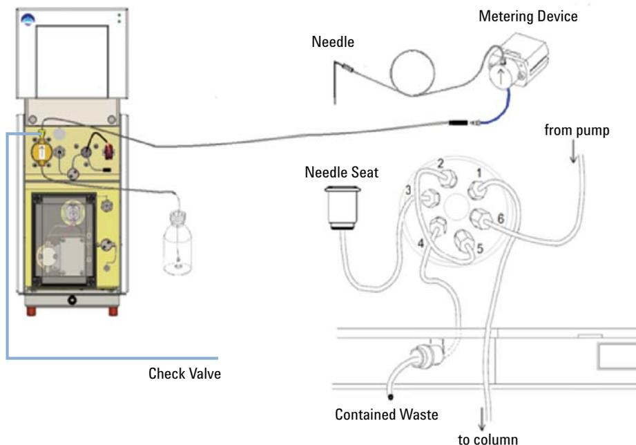
**Figure 22** Autosampler Fluidic connections
