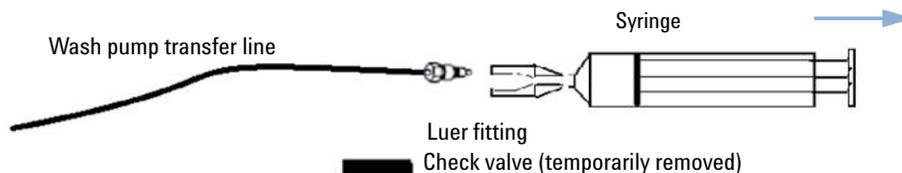
**Figure 14** Priming the wash line
