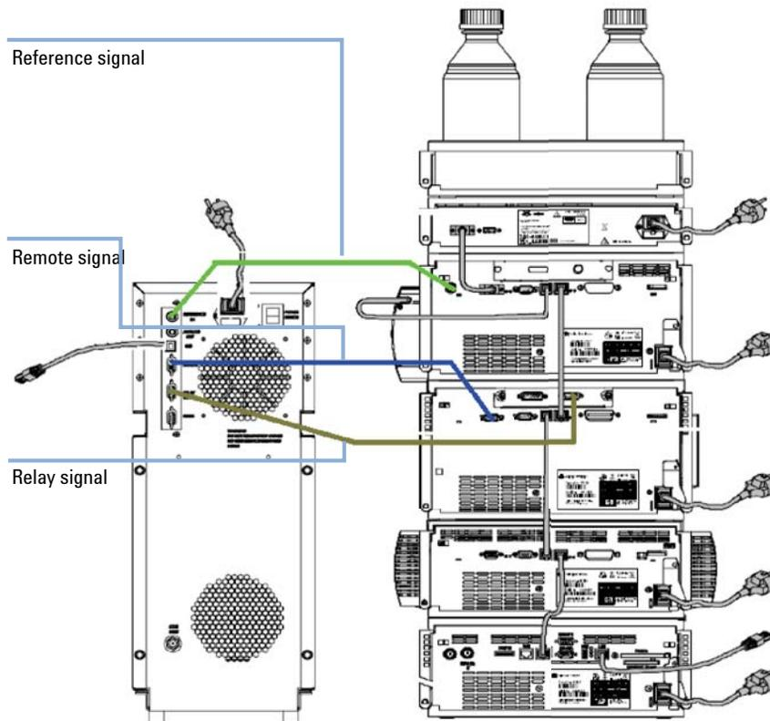
**Figure 16** Reference, Remote and Relay Signal Connections
