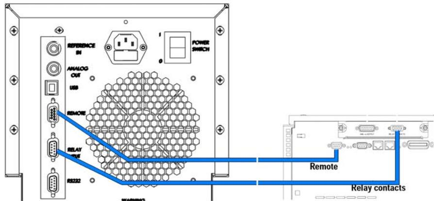
**Figure 24** Autosampler Signal Cable Connections
