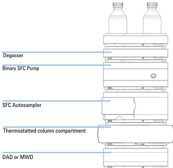
**Figure 18** Preferred order of Agilent HPLC Components
