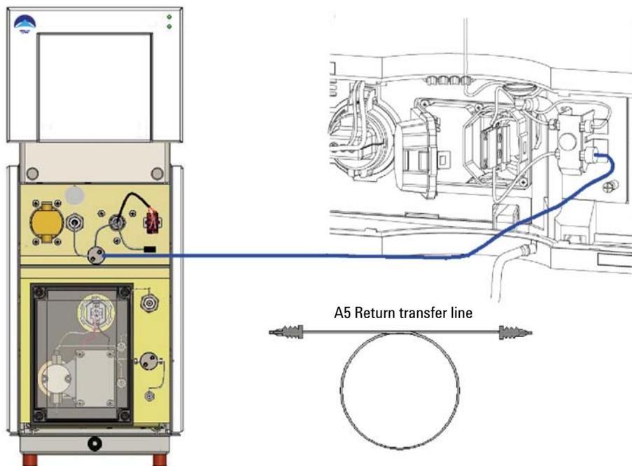
**Figure 8** Connecting the Aurora SFC Fusion™ A5 return Line
