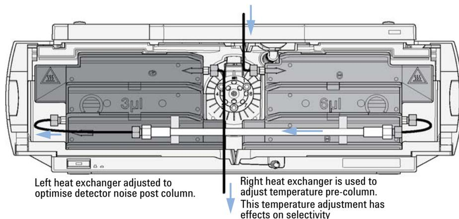
**Figure 9** Plumbing the Agilent 1290 Infinity Thermostatted column compartment
