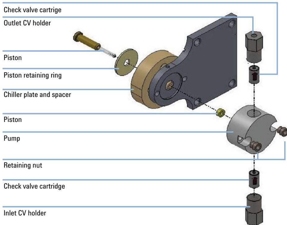
**Figure 30** Exploded view of Booster Components
