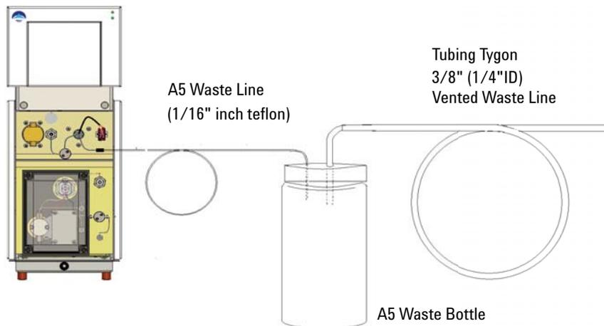
**Figure 6** Installing the Waste Container
