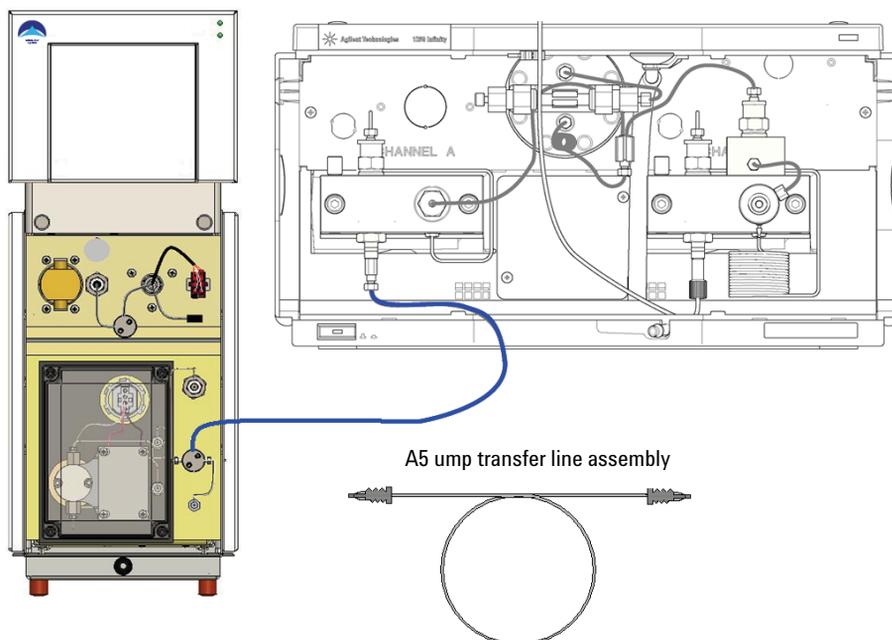
**Figure 11** Connecting the Booster outlet line
