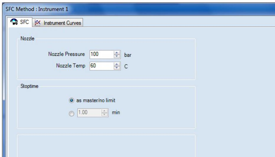
**Figure 29** Editing the Aurora Fusion A5 Method Parameters
