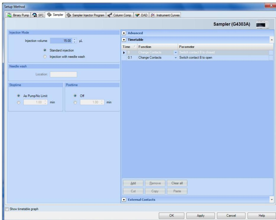
Default Pump setting is 80 %  $\text{CO}_2$  : 20 % modifier. Typical Flow rate in SFC is 3 mL/min; however, when SFC\_DEF.M is loaded, the flow rate is set to 0 mL/min. Solvent compressibility should be always set to **no compensation** for the  $\text{CO}_2$  Channel, and to the corresponding value for the modifier.
