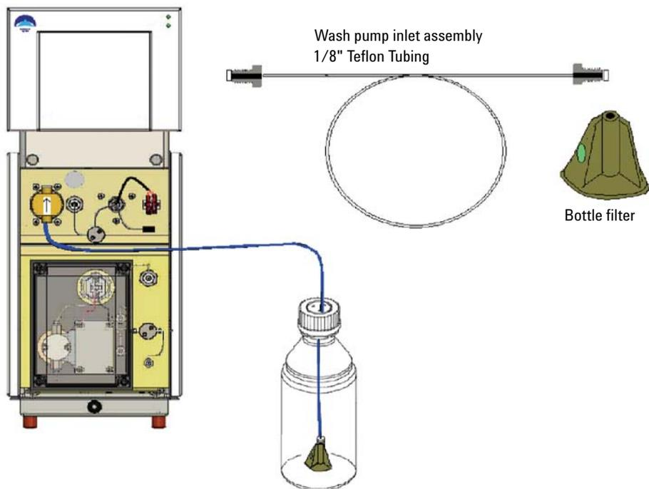
**Figure 12** Connecting the wash pump inlet
