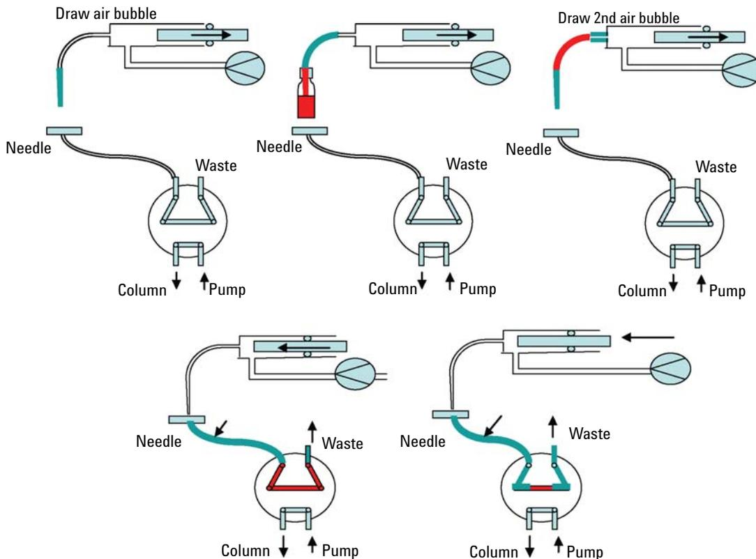
**Figure 26** Partial Loop Injection
