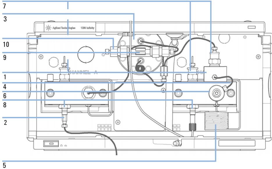
**Figure 31** Agilent 1260 Infinity SFC Binary Pump specific SFC Parts
