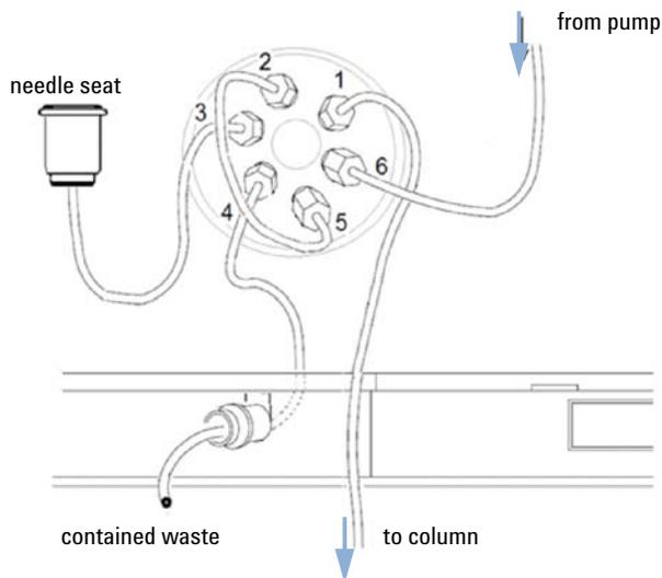
**Figure 10** Plumbing the G4203A SFC Autosampler
