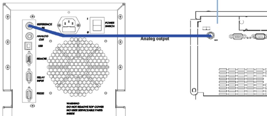
**Figure 20** Connecting the Analog Reference Signal
