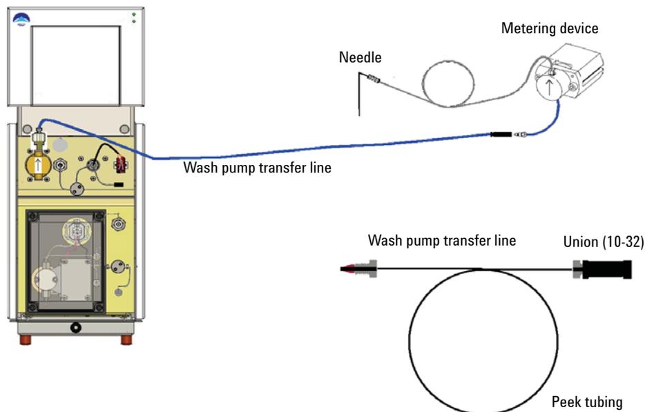
**Figure 13** Connecting the Wash Line and Check Valve
