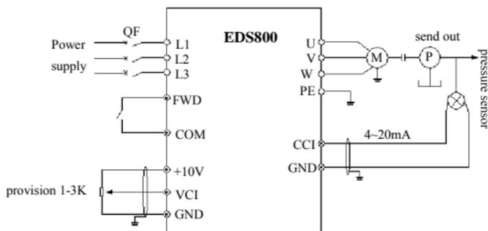
Fig.6-13 built-in PID analog feedback control system graph
