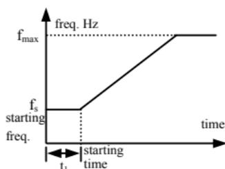
Fig.6-6 starting freq. and starting time
