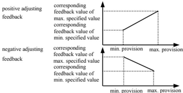
**Fig.6-16 provision, feedback curve**
