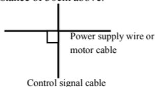
**Fig.3-16 system wiring demand**
