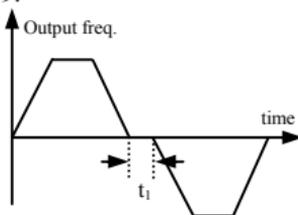
**Fig.6-9 FWD REV run dead-section time**
