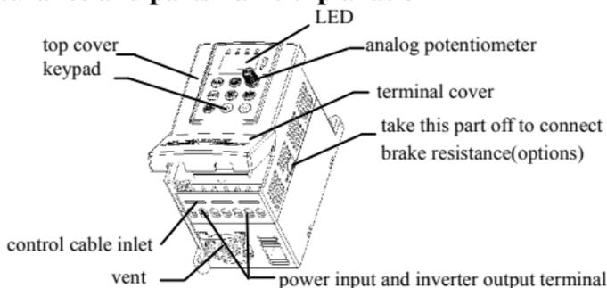
Fig. 2-3 Parts name sketch for EDS800
