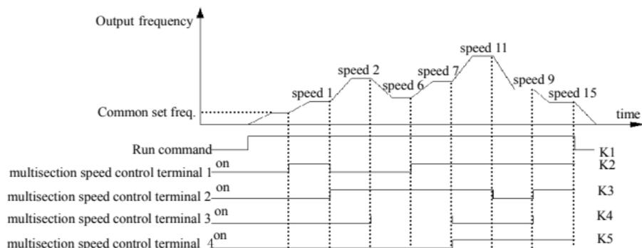
Fig.6-24 multi-step speed run
