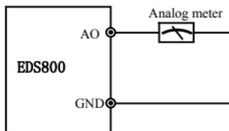
**Fig.3-10 analog output terminal wiring**
