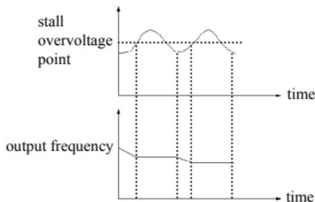
**Fig.6-38 overvoltage stall function**
