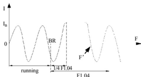
Fig.6-7 Zero freq. DC braking Volt. And Time
