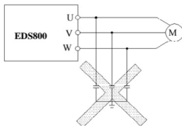
Fig.1-2 capacitor at output side forbidden
