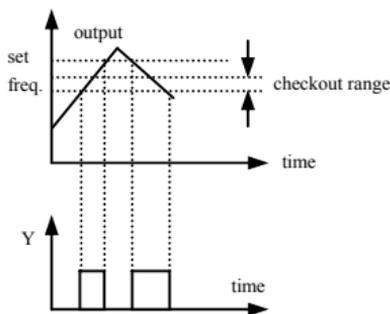
Fig.6-32 freq. arriving signal output
