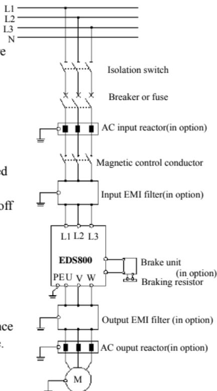
Fig.3-5 connection of inverter and fitting parts
