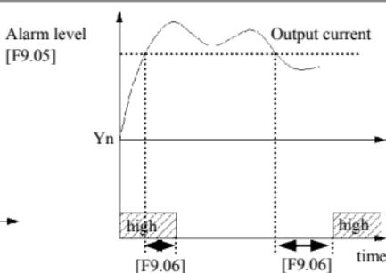
**Fig.6-36 electronic thermal relay protection** **Fig.6-37 overload alarm**
