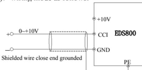
**Fig.3-9 CCI terminal wiring diagram**
