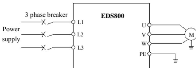
Fig.3-4 main loop simple wiring
