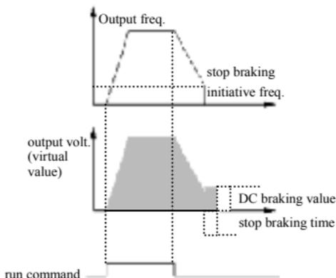
Fig.6-8 Dec stop+DC braking
