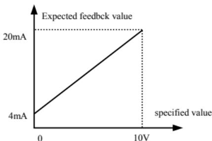
**Fig.6-15 specified value and expected feedback value**
