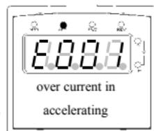
Fig.4-4 failure alarm
