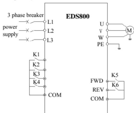
Fig.6-25 multi-step speed run
