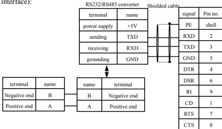
**Fig. 3-12 RS485 communication wiring**
