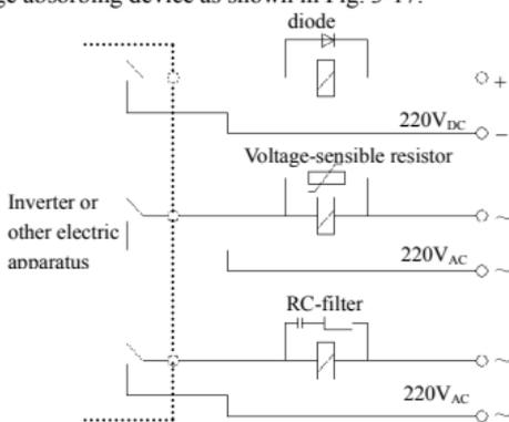
Fig.3-17 installation demand for electromagnetic on-off device
