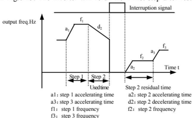
**Fig.6-23 PLC starting mode 1**
