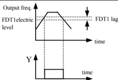
Fig.6-33 freq. level detecting
