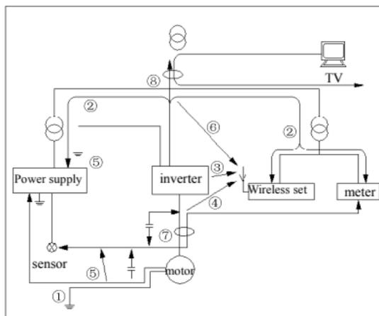
Fig.3-15 noise disturbance spread road sketch
