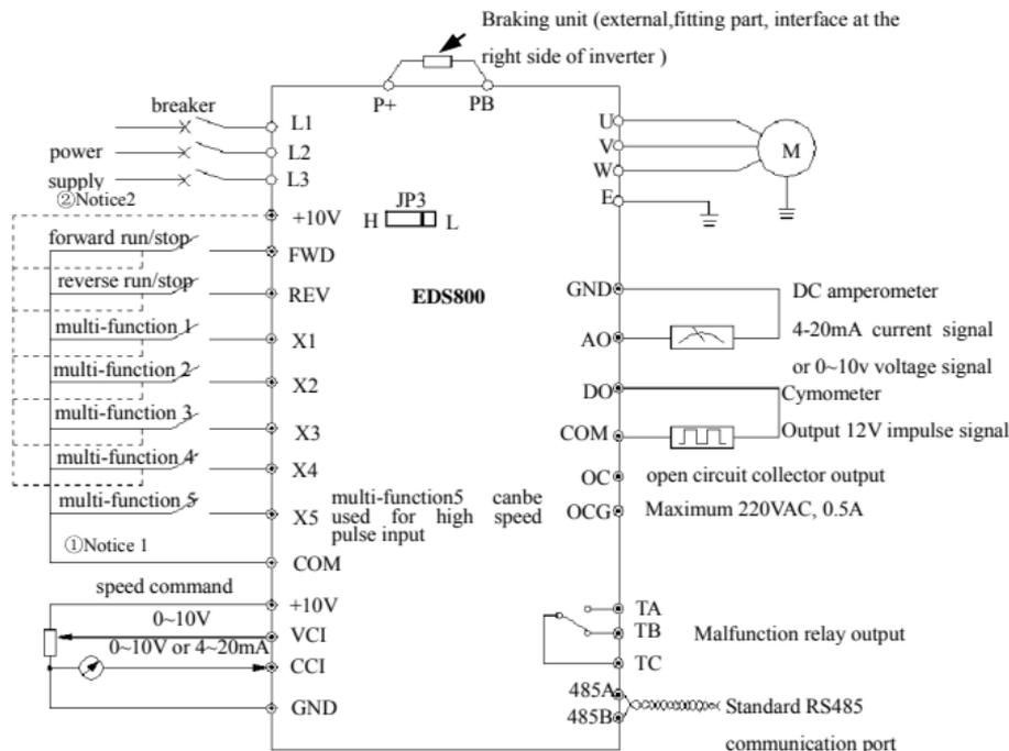
Fig. 3-6 basic wiring diagram
