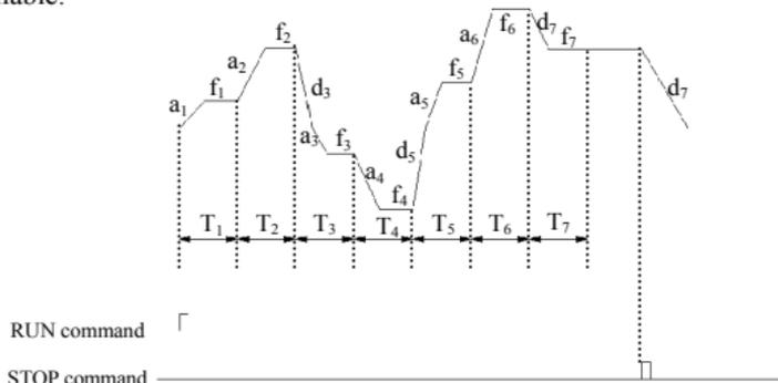
Fig.6-21 holding mode after PLC single circle
