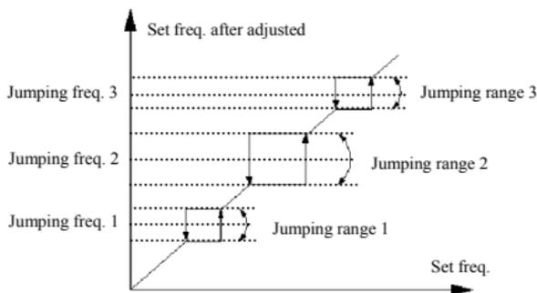
Fig.6-12 jumping frequency and range graph
