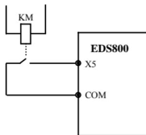
Fig.6-26 exterior device failure always-open input
