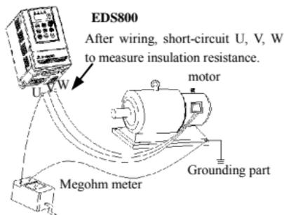
Fig.1-1 motor insulation measure
