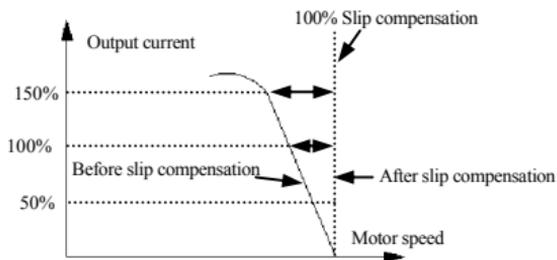
**Fig.6-10 slip freq. compensation graph**
