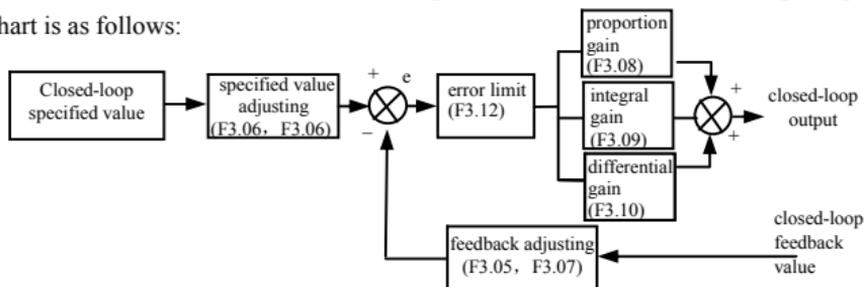
Fig.6-14 PID control principle diagram
