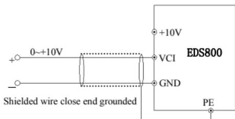
**Fig.3-8 VCI terminal wiring diagram**
