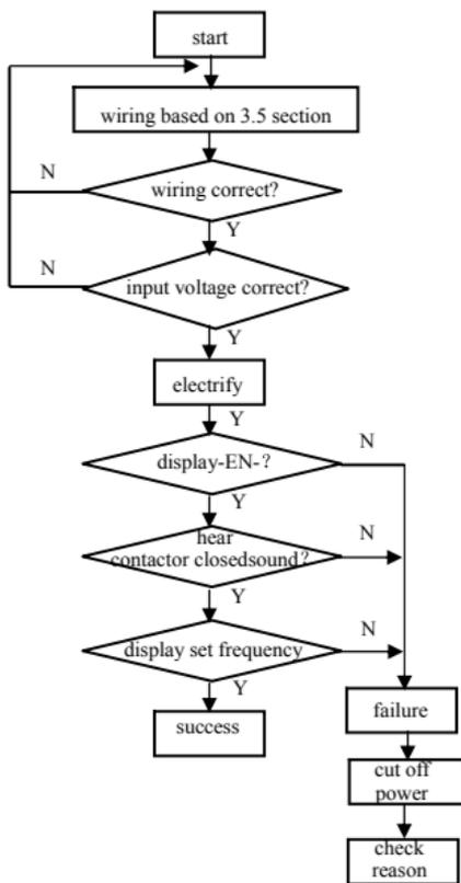
Fig. 4-12 first electrification operation flow
