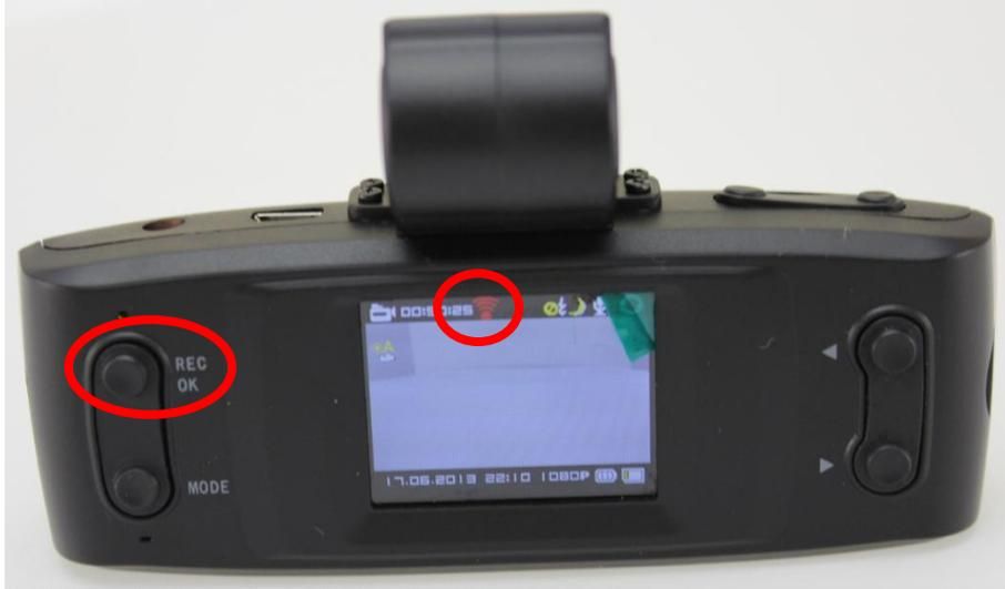
If you want GPS information while you are recording, wait for the symbol directly to the right of the recording time to turn green. This indicates that a GPS is receiving a signal. If it fails to turn green, try moving to an area where nothing is above you (you may have to take the device outdoors to get a signal). It may still take a minute or two to make the connection.
