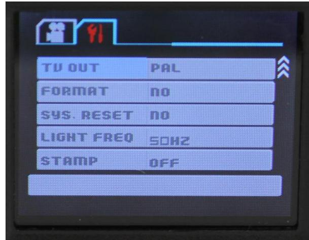
You can get to the settings menu by pressing MODE until you reach a screen with a screwdriver and wrench at the top of the screen. Press ► until you reach TV OUT, and you can press OK to select it. You can select the option you want using the ► and ◀ buttons and use OK to confirm the selection.
