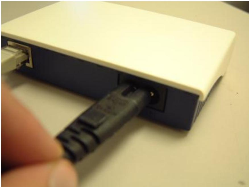
Plug your power connector of your power cable into the **power connector** at **the back** of the HomePlug Turbo Ethernet Bridge
