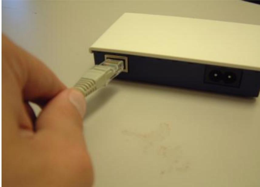
Plug **the other end** of your network cable into the **RJ-45 port** locate at the **back** of the HomePlug Turbo Ethernet Bridge
