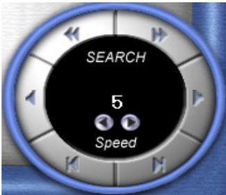
: Buttons in upper line works for fast rewind (left directional arrow) and fast forward (right directional arrow). Buttons in middle line activate the normal playing back in forward and reverse but the speed can be adjusted by controlling (-), (+) tap on the top. The buttons in lower line give playback frame by frame, forward or reverse.
