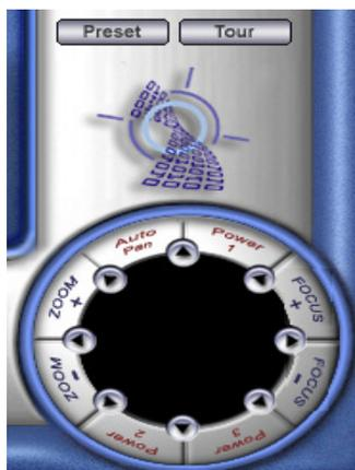
: PTZ cameras connected to DVR System can be controlled from DVR Multi Client. The arrow buttons will move the camera in the direction of the arrow, and the ZOOM, FOCUS buttons will manipulate the camera accordingly. However, only user with permission can control the PTZ setting.
