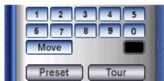
: When the PTZ camera supports preset function and tour, this control is available at DVR Multi Client. However, settings of preset and tour must be made at DVR System. And No. of available preset points are depending on the camera's feature.
