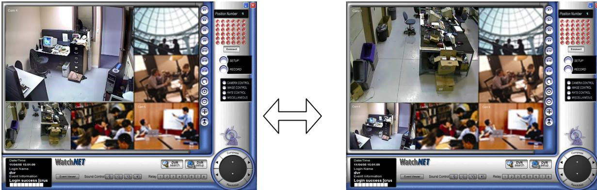
At the connection of Multi-client software, connected cameras will be positioned in order of camera numbers. It is possible to relocate the camera position to the desired location by left click on the image that needs to be relocated, drag it to the new position, and release the mouse button.
