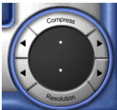
: Compression Rate can be adjusted between 10 ~ 90 to enhance the transmission speed (\* for default compression rate). Lower value will provide faster transmission. Resolution can be selected among 1/2, 1/4, or 1/8 (\* for default resolution), and lower resolution provides faster transmission speed. Compression rate and resolution adjusted here are not changing actual resolution and compression rate recorded on the server.
