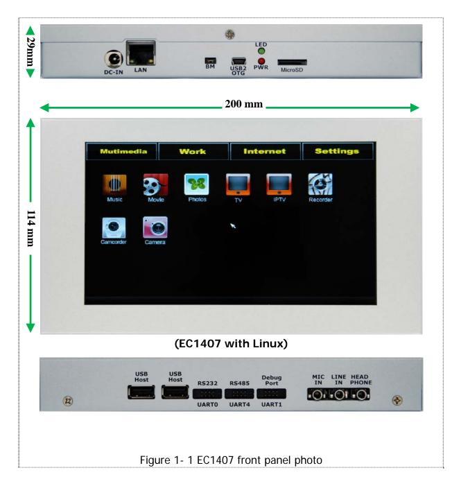
NOTE: EC1400 dimension is the same as EC1407, except that EC1400 has no front panel.
