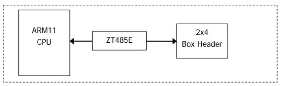
ZT485E: RS485 transceiver. RS485 works in half duplex mode.
