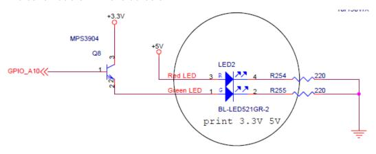
On EC1403/EC1404, the red and green LEDs are connected to user programmable GPIO\_E14 and GPIO\_E16:
