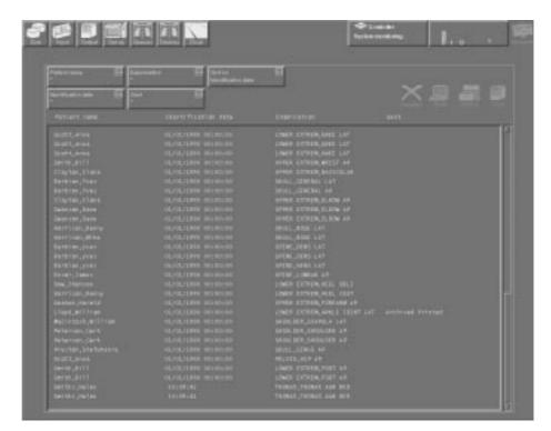
The images displayed on the alphanumeric image list are selected by default in accordance with the selection criteria that have been configured in the Setup module of the system main screen. In the example screen above, the preconfigured selection criteria are 'Patient name', 'Identification date', 'Examination' and the 'Sent' feature.
