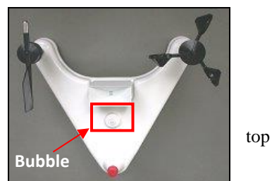
Figure 26: The bubble level confirms the station is level, which is required for accurate rainfall and solar radiation measurements.
