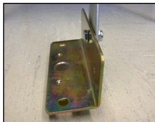
Figure 17: For temporary sites, drive the stakes of the TP1-ST Kit (left) through the center hole in each tripod foot (right). The stakes should be driven in until they barely contact the foot surface. For permanent sites, install user-supplied bolts through the holes in each tripod foot.
