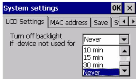
“LCD Settings” page of the **cecp** provides the function to turn off the LCD backlight, and thus elongates the period of service. For example, if the user wants the backlight turned off automatically after 10 minutes when the device was no longer used. The user must select “10 minutes” in the put down box and then press “OK” button. Then the screen save function is enabled. Once the backlight was turned off, events or perturbations from the touch screen can turn it on.
