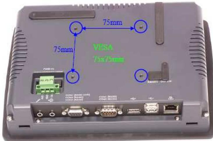
The NP-880S VESA Standard hole for wall mounting or arm mounting. The M4 screw length is 10 to 15mm. Don't over 15mm. The CPU board will damage.
