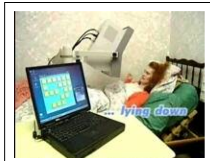
Figure 2.1. When used in combination with a hydraulic base, the Visioboard mounting system is sufficiently flexible to enable it to be positioned for use by someone lying down.
