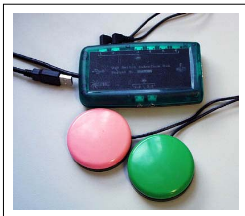
Figure 2.18. Example of switches and switch interface – depending on the user's preference and ability, switches can be operated by many different parts of the body (eg. head, hand, knee, etc.) in combination with the eyes to emulate full mouse control.
