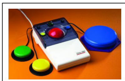
Figure 3.4. Illustration of robust special needs trackerball with switches to emulate mouse button features.
