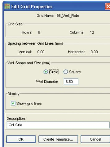
The grid size and spacing are listed in the Properties for information only. To change the number of rows or columns in a grid, you must delete the grid, change the Grid Template settings, and apply the grid again. Grid spacing can be changed by reshaping the grid as described above in *Resizing A Grid*.
