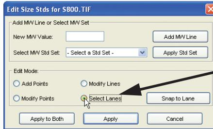
With the edit mode set to **Select Lanes**, you can click on the centerline of a lane to select it. Additional standards lanes can be selected by holding down the **Control** key and clicking the centerline of the lane. All lanes with standards should be selected and there should be no sample lanes selected. If you have trouble selecting a lane because the center-line is covered with band markers, click near the top or bottom of the lane.
