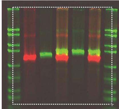
When the mouse button is released, the specified number of lanes is placed on the image. Lane width is determined by the Application settings. Bands are automatically found and enclosed by a band marker after the lanes are created.
