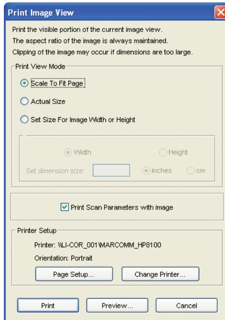
Scan parameters (resolution, etc.) can be printed with the image by selecting **Print Scan Parameters with Image**. Click **Page Setup** if you want to select portrait or landscape page orientation. To change printers before printing, click **Change Printer**.
