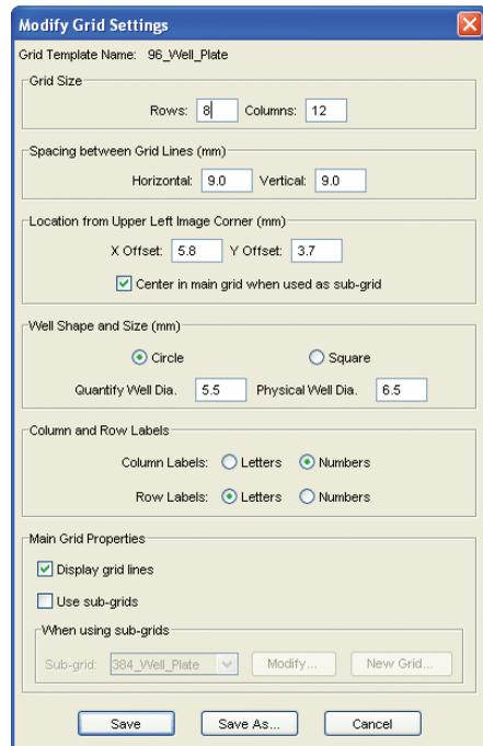
**Grid Spacing:** The vertical and horizontal spacing (in mm) of the grid lines can be changed in order to match the spacing between objects on the image. The vertical and horizontal spacing should be the same as the vertical and horizontal center-to-center distance between objects on the image. See *Measuring Size and Distance on the Image* below.
