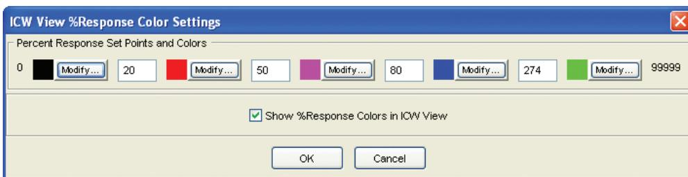
Each color can be changed by clicking the corresponding **Modify** button. The response range associated with each color can be changed by typing a new integer for the upper limit in the appropriate field. The lower limit of the range is always the upper limit of the previous range.
