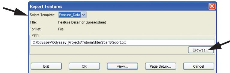
Templates that produce data files export the data to a plain text file. Each line in the file represents one feature or lane. On each line, the fields designated in the template are separated by the field separator character specified in the template. To set the path and file name for the data file, click the **Browse** button.
