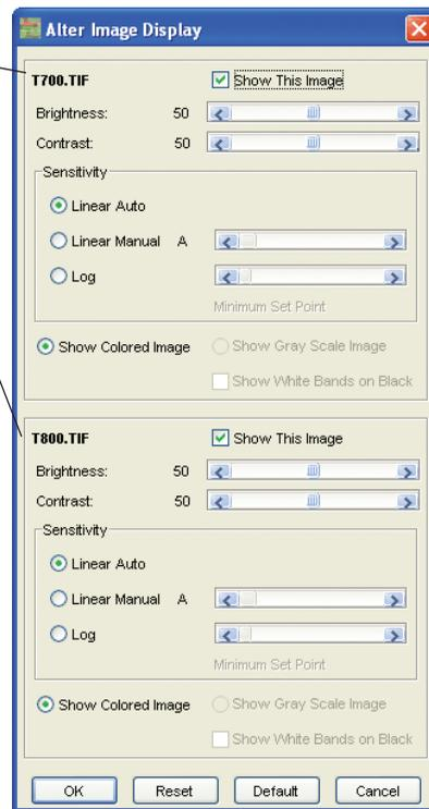
Each image has its own set of **Brightness**, **Contrast**, and **Sensitivity** sliders. The **Brightness** and **Contrast** sliders change the appearance of the background and bands in the image.
