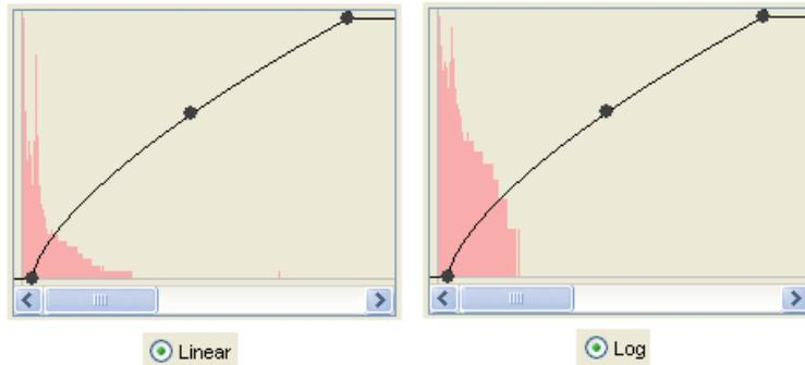
The X-axis of the histogram can be expanded or contracted using the **Contract/Expand** slider. The scroll bar underneath the histogram can be used to scroll along the X-axis. When the X-axis is expanded, the **Min Pt.**, **Cntr**, and **Max Pt.** buttons can be used to quickly scroll to the minimum point, midpoint (center), and maximum point, respectively.
