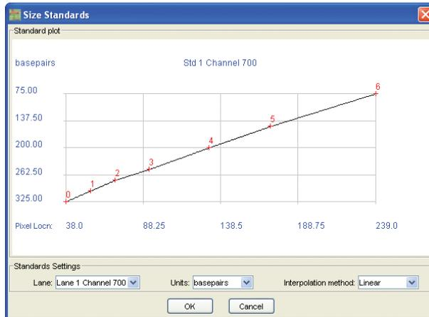
Selecting the correct interpolation method is important because it affects the size assigned to sample bands. **Linear**, **Log**, **Reciprocal Fit**,
