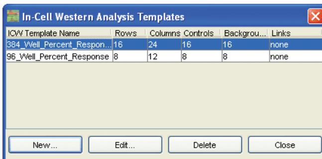
The In-Cell Western Analysis Templates window lists all current templates and a few of their distinguishing parameters. To edit or delete a template, select the template in the list and click the **Edit** or **Delete** button, respectively. To copy a template, select the template, click **Edit**, change the template as needed, and click **Save As** to save the template under a different name.
