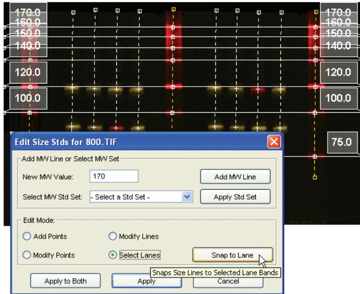
When lines are snapped to the bands, control points are added and MW lines are drawn as described above for MW standard sets. After the MW lines are snapped to the bands, the lines must be applied to the image using the **Apply to Both** or **Apply** buttons (see *Applying Standards to the Image* above).
