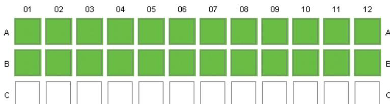
Select **Link Rows** and click **Create Link**. The green wells in the template turn black to indicate they are linked. Each individual link (A01-B01, A02-B02, etc.) is listed in the **Existing Links** list. During analysis, the linked wells in the **Existing Links** list will be averaged. The average will be used in ICW calculations rather than individual integrated intensity values. Only sample wells are averaged. (All **Background** and **100% Standard** wells are always averaged.)
