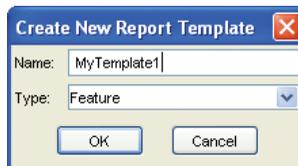
Enter a name for the template in the **Name** field. Templates should be named using a convention that makes them easy to distinguish in a list. When the default templates were created, *\_Print* or *\_Data* was appended to the template names to indicate whether the new template was a printing template or a data output template.
