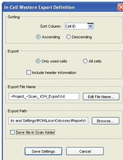
You can determine how the data are arranged in a report by choosing the column on which to sort and whether the data should be sorted in ascending or descending order. In the **Export** section, you can choose to output data for all cells in the table or to exclude cells that are marked as empty wells in the microplate. When **Include Header Information** is selected, information about the project, scan, and analysis is included in the beginning of the file.
