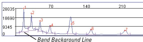
Displaying the band background line can be useful if you are quantifying bands in lanes and you are trying to determine whether to use the band background or the lane background in the background calculation (see Chapter 8).
