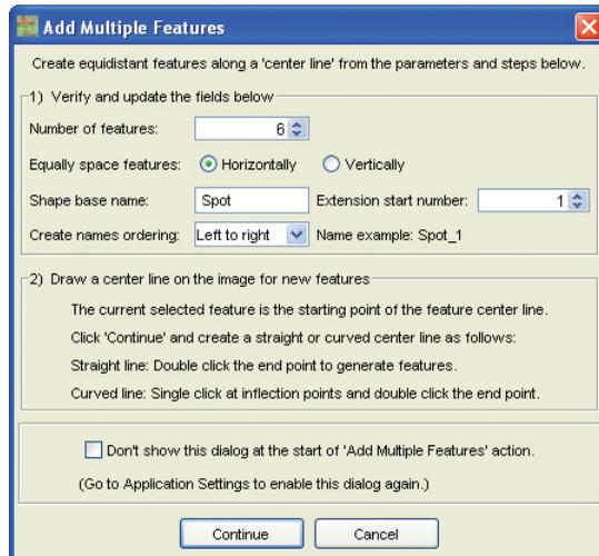
In the Add Multiple Features window, start by specifying the number of features to add and whether the features should be spaced equally in the horizontal or vertical dimension. Features are named with a prefix (base name) and a numbered extension (see **Name Example** in the window above). Name extension numbers are incremented for each feature, moving in the specified direction: left-to-right, right-to-left, top-to-bottom, or bottom-to-top.
