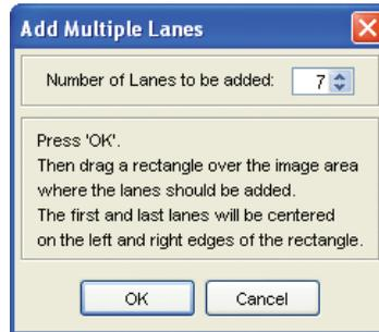
After clicking **OK**, click and drag a rectangle over the image area where the lanes should be added. Start in the center of the first lane, at a height that will correspond to the upper lane boundaries.
