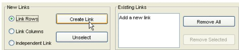
Additional links between wells with identical samples can be added by continuing to select the wells and click **Create Link**. If you need to link columns rather than rows, click **Link Columns** rather than **Link Rows**. If you don't want to link entire rows or columns, select the wells, click **Independent Link**, and click **Create Link**.
