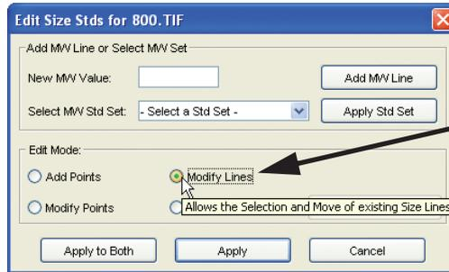
Click a MW line to select it and move the cursor over the line until it becomes an up-down arrow cursor as shown below.
