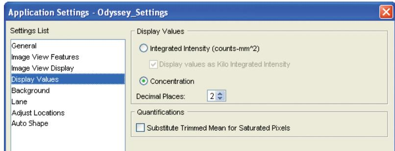
Quantification values are displayed as integrated intensity when **Integrated Intensity (counts-mm<sup>2</sup>)** is selected. Clicking **Concentration** displays values in Concentration units. The number of decimal places used when the concentration value is displayed can be changed using the **Decimal Places** field.
