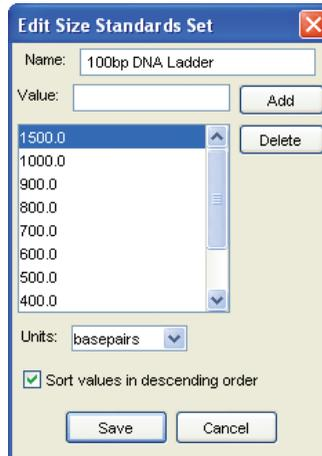
Begin by selecting the units for the set using the **Units** drop-down list. Basepairs, kilobasepairs, daltons, and kilodaltons can be selected.
