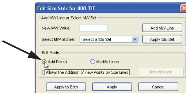
Click on a MW line at a position where an inflection point needs to be added. Any line can be clicked and any number of points can be added by continuing to point-and-click, as long as the Edit Mode is still set to **Add Points**. To stop adding points, switch to one of the other edit modes like **Modify Points**.
