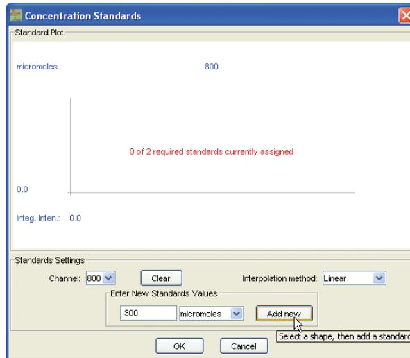
First, make sure the **Channel** (700 or 800) matches the image you are analyzing. Next, enter the concentration for the selected standard in the **Enter New Standards Values** field, select the units, and click **Add New**.
