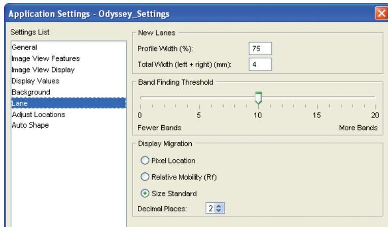
Application settings for lanes are used to control the characteristics of a lane when it is first created. Adjusting the Application settings for lanes can increase band finding accuracy and make the initial lane boundaries more closely match the lanes in the image.
