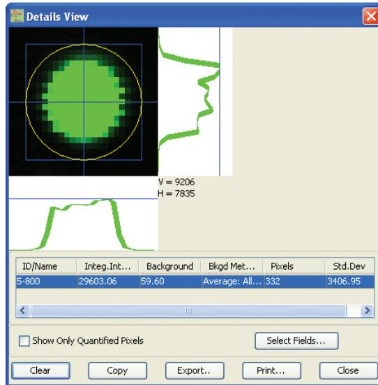
Details View shows an enlarged view of the dot/band along with the shape that surrounds it. The center of the feature surrounding the dot/band is marked by the blue cross hairs. The sides of the blue rectangle are the horizontal and vertical boundaries of the feature on the image. In the case of a rectangle feature, the blue line actually represents the rectangle. The curves to the right and below the image plot the intensity of the pixels below the cross hairs.
