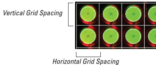
**Offset From Upper Left Image Corner:** These X and Y coordinates determine the placement of the upper left corner of the grid. The offset, in millimeters, is measured from the upper left corner of the image.
