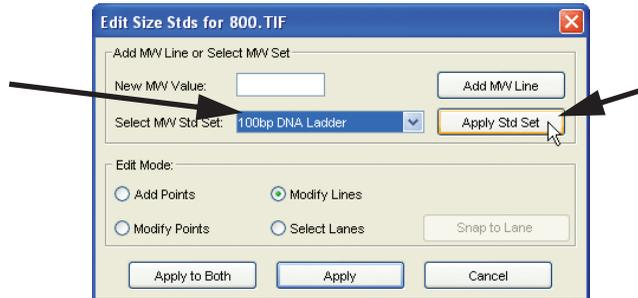
MW lines for all standards in the set are added to the image at once when **Apply Std Set** is clicked. The next step is to identify which lanes contain standard bands and then automatically match the MW lines to the bands in the standards lanes.
