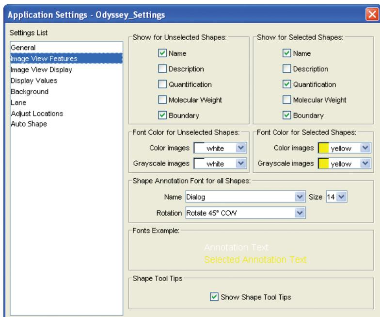
The Image View Feature settings can be used to reduce the "screen clutter" that can occur when labels are displayed on closely spaced features. Notice that there are two groups of settings – those for
