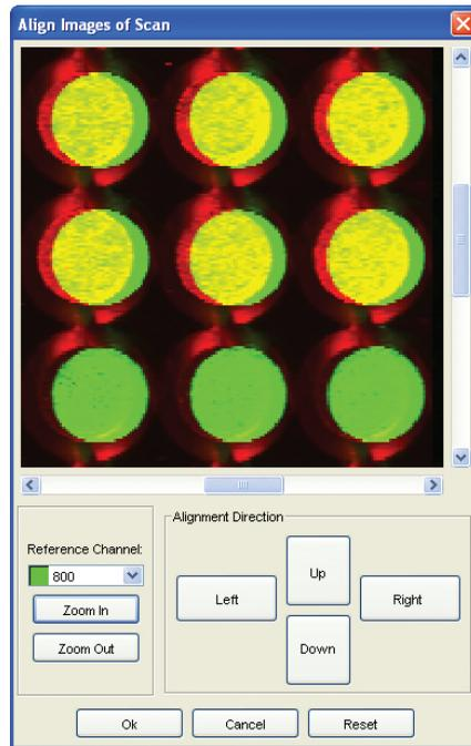
To correct an offset, start by using the zoom buttons to make the offset clearly visible. Next, select the reference channel that stays stationary while the other channel is moved. Last, move the channel not designated as the reference using the **Alignment Direction** buttons. The **Up**, **Down**, **Left**, and **Right** buttons move the image one pixel at a time. If you make a mistake and want to start over, click **Reset**.
