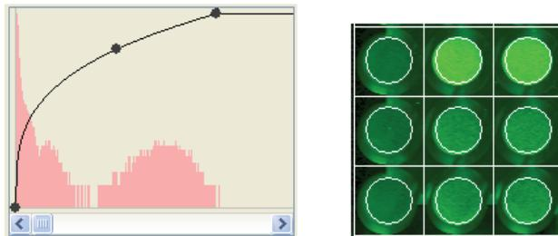
The midpoint can be dragged in only the vertical dimension. As the midpoint is moved, the shape of the adjustment curve is changed, which results in dark pixels and bright pixels being adjusted by different amounts. In general, changing the midpoint will have the greatest impact on the mid tone pixels, but the bright and dark pixels will also be changed.
