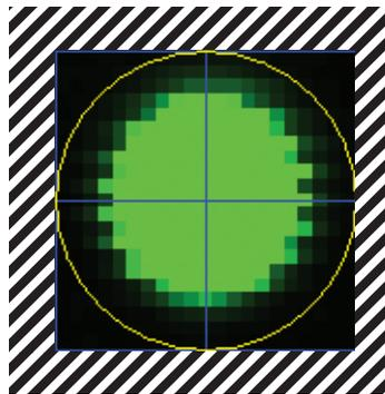
*To illustrate the location of the pixels used for Average or Median background methods, the pixels have been covered with diagonal lines.*
