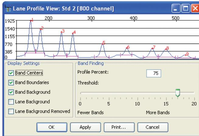
The title bar of the lane profile indicates which lane is profiled and the image on which the lane is located. If you open lane profiles with channels overlaid, two profiles are opened – one for the lane in the 700 channel and one for the lane in the 800 channel. Similarly, if more than one lane is selected, profiles will be opened for all selected lanes.
