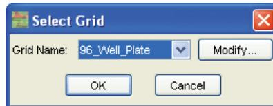
If you need to change the grid template before applying it, click the **Modify** button in the Select Grid window and change the grid parameters as described above under *Grid Parameters*.
