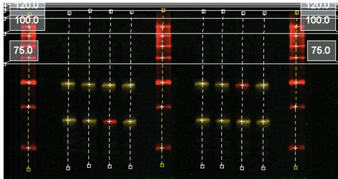
Click the **Snap To Lanes** button in the Edit Size Stds window to link the MW lines to bands in the standards lanes.
