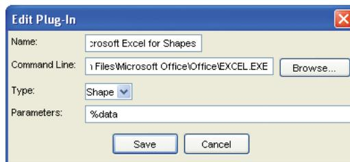
The **Command Line** should specify the program to start when the plug-in is launched. The program and path can be specified by clicking **Browse** and using the file selection window to find the program. Any program that accepts a data file parameter when launched from a command line can be used in the plug-in. If you intend to transfer data to the program, it must accept data separated by tabs, spaces, etc.
