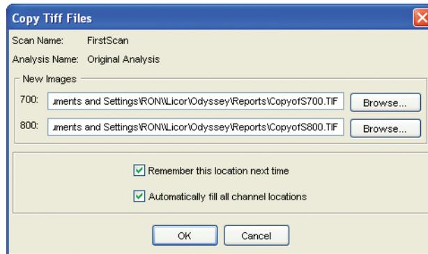
The **Browse** button opens a standard file selection window. If **Automatically fill all Channel Locations** is selected, the path for the second channel is automatically updated when the path for the first
