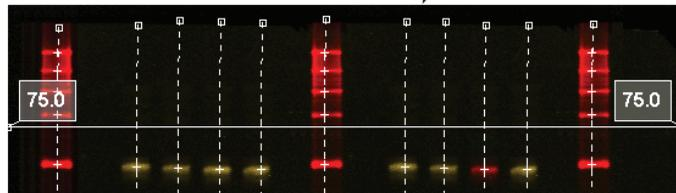
After clicking **Add MW Line**, a MW line is displayed on the image that will connect all the standard bands of a particular weight (75 bp in the example above). The MW line itself represents all the points of equal MW on the gel. The placement and shape of the line is not important yet. After the first line is added, add the rest of the MW lines by entering their MW and click **Add MW Line** as described above.
