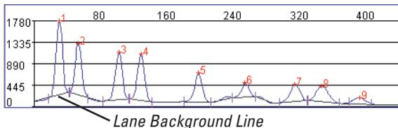
The lane background line is calculated by selecting appropriate minima points from the lane profile. Displaying the lane background line can be useful if you are quantifying bands in lanes and trying to determine whether to use the lane background or band background in the background calculation (see Chapter 8).
