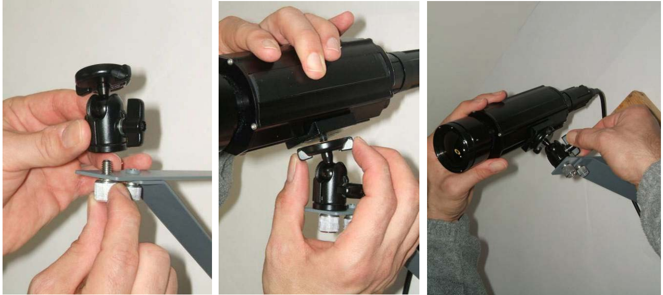
Figure 13: Attaching the Tripod Ball Head and Thermal Camera
