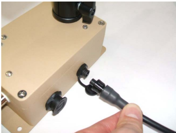
Figure 8: Attach Power and Data Cables to DOG Camera Unit
