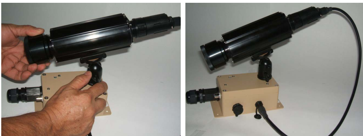
Figure 19: Adjusting Thermal Camera Rotation and Tilt
