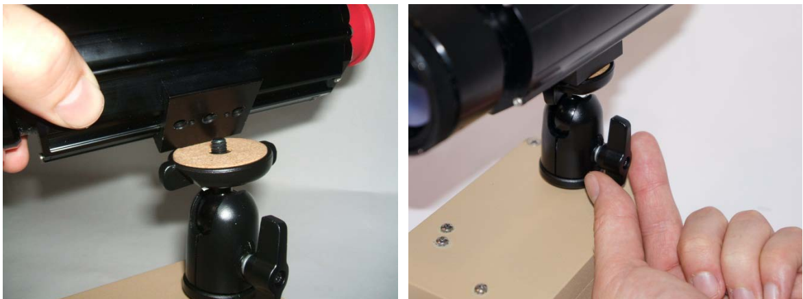
Figure 6: Attaching and Adjusting the Thermal Camera to DOG Camera Unit
