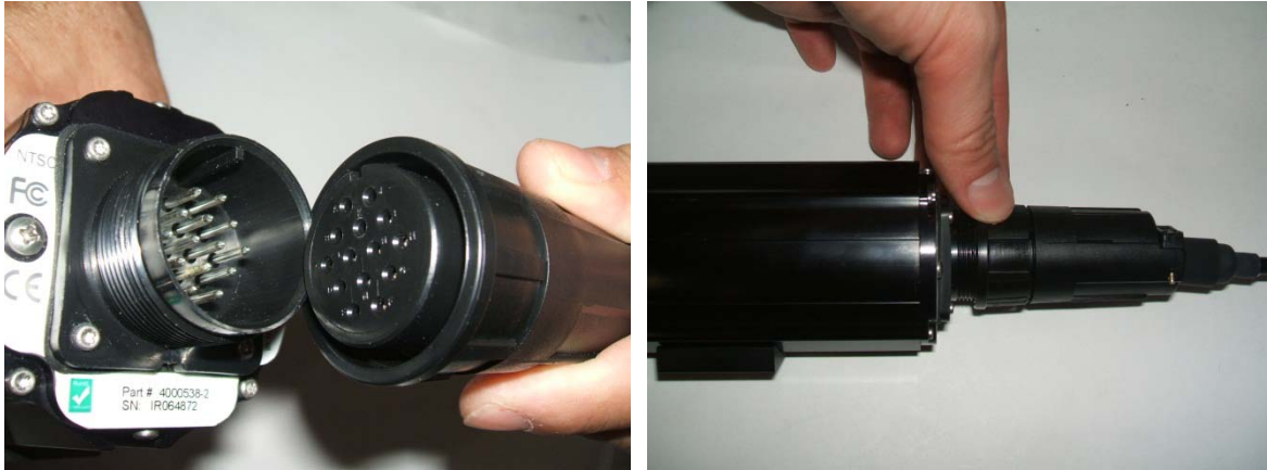
Figure 16: Attaching 14-Pin Circular Connector to the Back of the Thermal Camera
