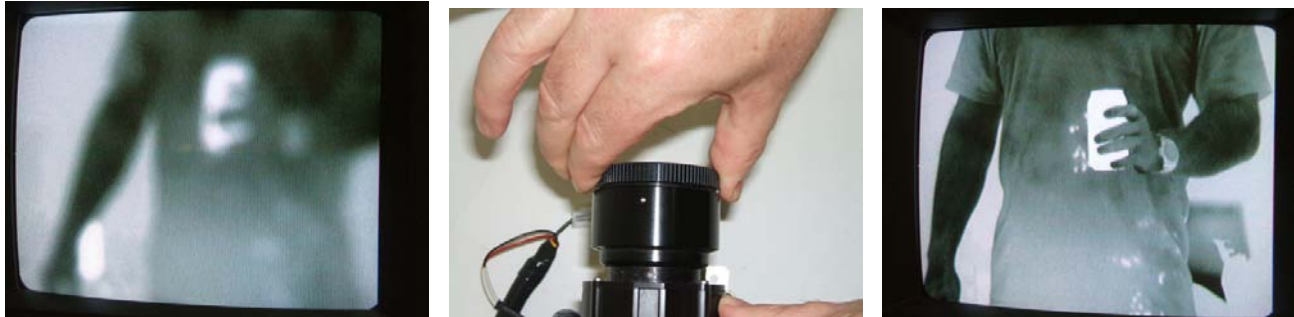
Figure 20: Focusing Thermal Camera
