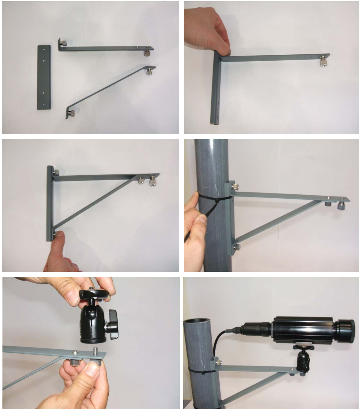
Figure 15: Pole Mounting Procedure
