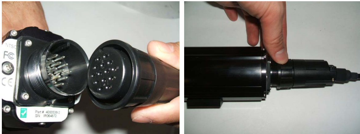
Figure 7: Attaching 14-Pin Circular Connector to the Back of the Thermal Camera
