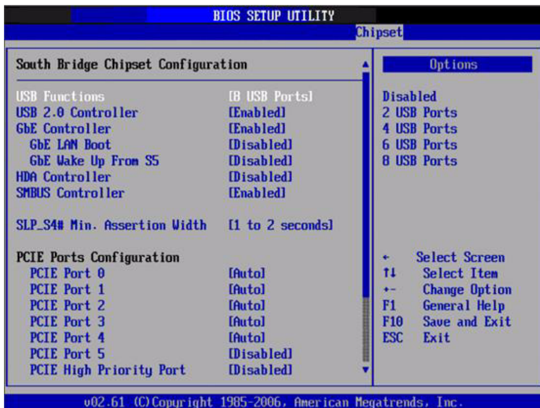
Figure 3.27 South Bridge Configuration
