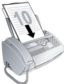
3 Then configure the desired resolution. You can choose between **RESOL. : STANDARD** (for documents without special features), **RESOL. : FINE** (for texts with small print or drawings) and **RESOL. : PHOTO** (for photos). Press **RES**. The configured resolution ap-
