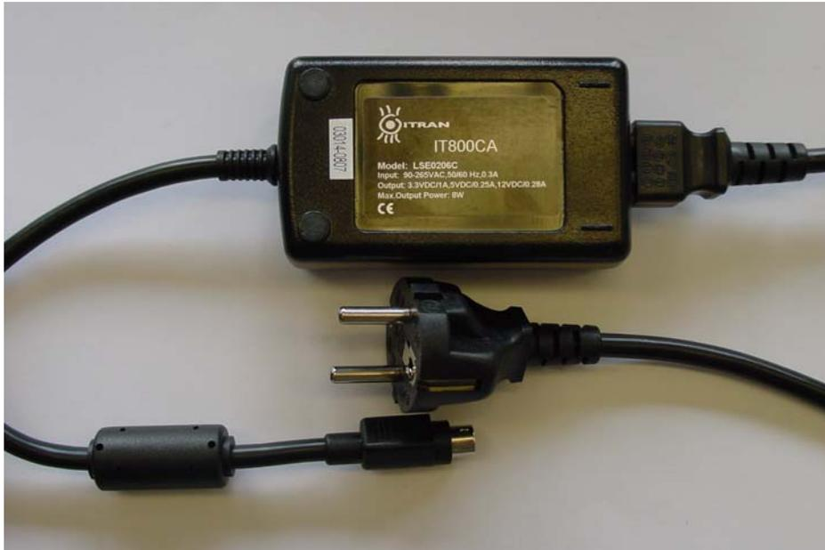
**Figure11: The YITRAN power supply including line coupler**
