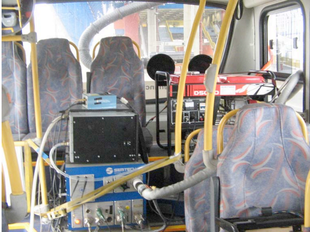
Figure 3b: Interior of a Bus Outfitted for Emissions Testing
