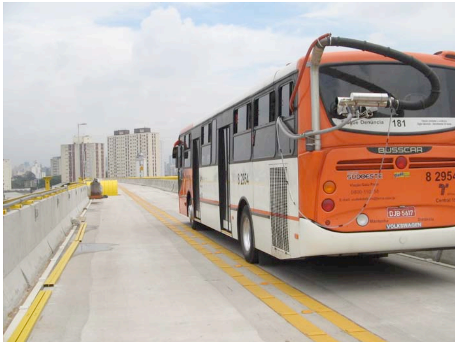
Figure 3a: Exterior of Bus Outfitted for Emissions Testing
