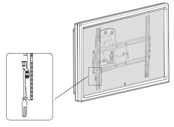
The lock designed feature can prevent your television from being removed from the crossbar. First, put the security lock in place, then tighten the bolt with screw driver by turning clockwise until tight (See illustration).
