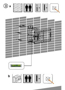
With the help of an assistant, and using the bubble level to ensure the wall plate is level, position the wall plate against the wall in the desired mounting location.
