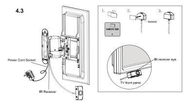
Plug mount power cord into power outlet. Attach IR Receiver to TV: Using the provided velcro tab, adhere the IR receiver eye-piece to the TV front panel so it has a clear line of sight with the remote control. (Fig. 6)
