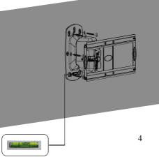
With the help of an assistant, and using the bubble level to ensure the wall plate is level, position the wall plate against the wall in the desired mounting location.
