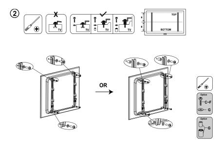
Attach the 2 TV arms to the back of your  $T^{3/2}$ . Typically your TV comes with the correct size screws, but we included a selection of the most commonly used screws.
