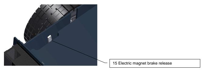
The wheels (7) are coupled to/disconnected from the motor by means of the handbrake button. If the handle is pulled down it is in the free position, the Multi-Mover S can now be freely manoeuvred by hand. If the button is pressed down, the Multi-Mover S can only be driven electrically.
