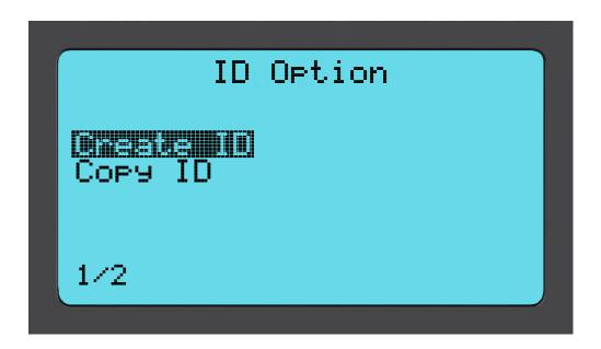
Selecting Copy or Create will prompt the user to place the correct sensor in front of the tool, and then the tool will program the sensor. The different sensors that can be programmed by the tool may have slightly different procedures, and may take slightly different times, but the prompts from the tool are clear.
