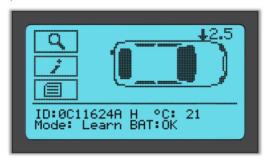
The arrow will then automatically move on to the next wheel position (Right Front, Right Rear and then Left Rear), and the pressure will be displayed against the previous wheel position, in Bar or PSI as selected in Settings.
