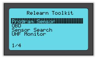
In this case the left front sensor has already been read, but needs to be replaced. After reading use the Down Arrow to navigate to the 'Relearn Toolkit' then 'Program Sensor' and select the programmable sensor you would like to use.
