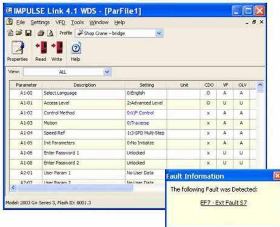
Or you can simply go to the Help Icon and go to the Drive Fault References for a complete list of P3 Series 2, G+/VG+ Series 2 and 3 drive faults, as shown below:
