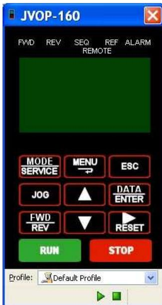
**Keypad Simulator** – The keypad simulator emulates the P3 Series 2 or Series 2 or 3 keypad which allows for remote keypad menu navigation. **This function is only available when IMPULSE• LINK 4.1 WDS is connected via the drive’s keypad 1CN connector (instead of the standard RS485 connection) – primarily for training purposes.** If you attempt to run the keypad simulator while connected via the standard RS485 connection a CF00 Comm Error will occur.
