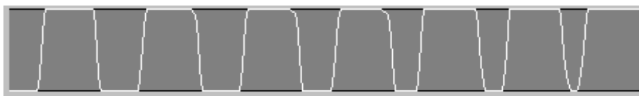
Figure 24 – Waveform with gain too high
