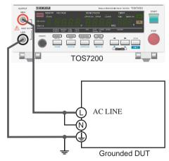
Fig.3-6 Connecting the Tester to a Grounded DUT (insulation resistance test across the AC LINE and chassis of the DUT)
