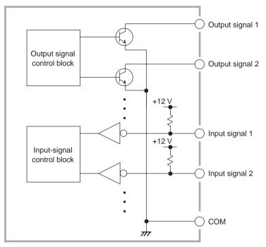
Fig.4-3 Internal Configuration of the SIGNAL I/O Connector
