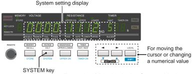
Fig.3-13 Example of Display in the System Mode
