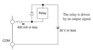
Fig.4-6 Example of Driving the Relay
