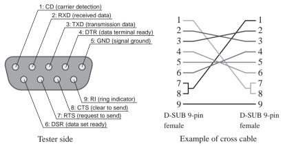
Fig.5-1 9-pin AT-type Connector
