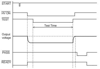
Fig.3-10 Example of the Timing Chart of PASS Judgment
