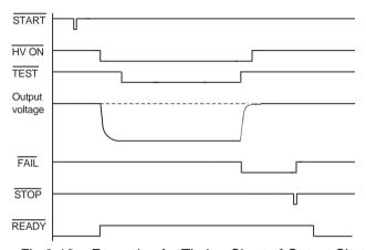
Fig.3-12 Example of a Timing Chart of Output Shutoff Caused by FAIL Judgment
