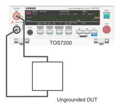
Fig.3-7 Connecting the Tester to an Ungrounded DUT
