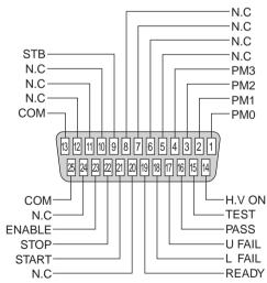
Fig.4-2 Pin Configuration for the SIGNAL I/O Connector
