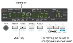
Fig.3-2 Setting the Test Voltage
