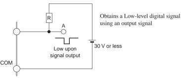
Fig.4-7 Example of Obtaining a Low-level Digital Signal
