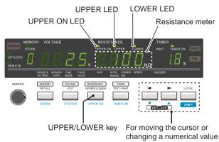
Fig.3-3 Setting a Lower Resistance
