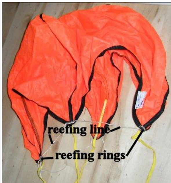
Parachute Skirt Reefing With Control Line.
