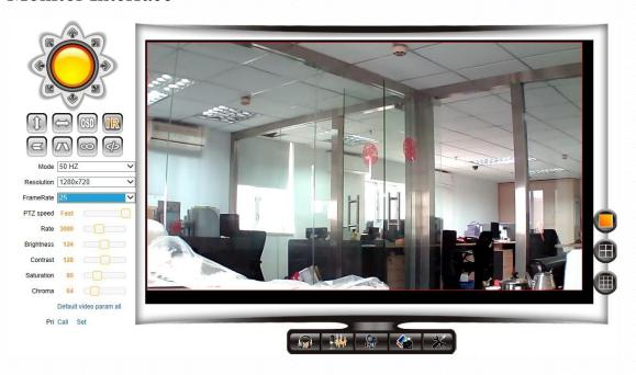
The camera will Left-right cruising automatically after select on, it will cruising about 1 hours if no manual stopped.Infrared light will be start work automatically in low-light condition. The number larger, the speed faster. Infrared light turn off in low-light condition. Image inversion: In selected, the image displaying will be upside down.Mirror image mode: In Selected, the displayed image will reversed left to right.
