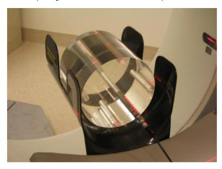
Note: Only one exposure with the probe in the center hole is required. The section "Theory of CTDI and k-factor" describes the theory behind this method.
