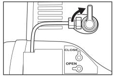
4. Close the drain cock and make sure no air is leaking from the cock.
