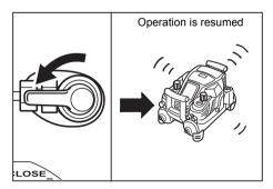
Discharge the compressed air by opening the drain cock somewhat. Make sure that the operation is resumed due to a decrease in the pressure.
