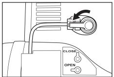
11. Open the drain cock to discharge all the compressed air and water in the air tank. If you found any abnormalities in the checkup or inspection prior to the operation, send the machine to your dealer or authorized service facility for inspection or repair.
