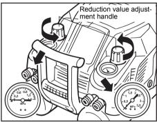
10. Turn the adjustment handle (in 2 locations) of the pressure-reduction valve counterclockwise to make sure that this turning moves the pressure gauge pointer downward at both locations. (You may hear sounds due to air leaking but it does not mean there is a failure.)
