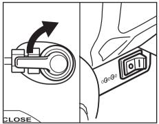
Close the drain cock and turn the power off while the compression operation is turned on to make sure that these actions stop the machine from operating.
