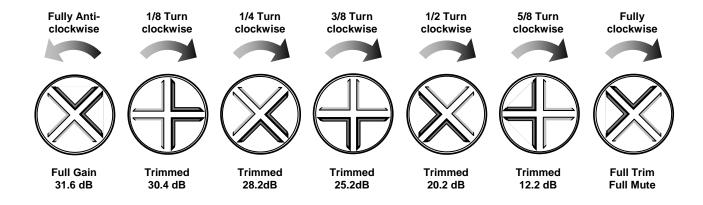
**NOTE:** These values and positions are approximate and should be used as a guide. During the installation and set-up, you should adjust the trimmer to achieve the desired output level.
