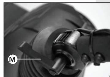
Folding down the steering
