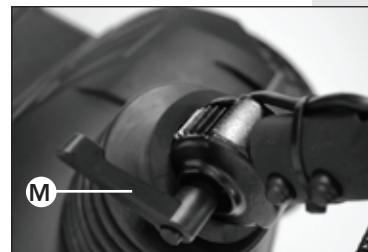
Change handlebar angle
