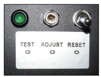
**RESET:** The new left-side control panel has three items. The toggle switch (reset) is a momentary closing switch, that has the same function as the reset button on the counter, but is more convenient for the operator.
