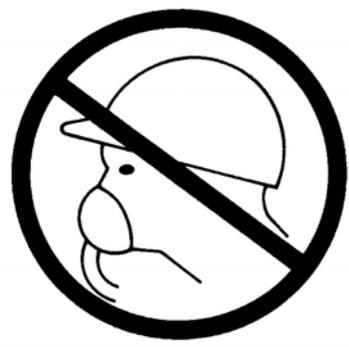
DANGER: AIR USED FOR BREATHING OR FOOD PROCESSING MUST MEET OSHA 29CFR 1910.134 OR FDA 21CFR 178.3570 REGULATIONS. FAILURE TO DO SO MAY CAUSE SEVERE INJURY OR DEATH.
