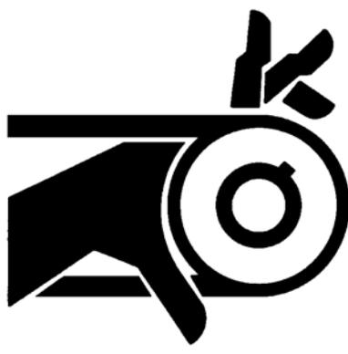
DO NOT OPERATE WITH BELT GUARD REMOVED. CAN CAUSE PERSONAL INJURY. EQUIPMENT MUST BE GUARDED IN ACCORDANCE WITH OSHA REGULATION CFR 1910.219.
