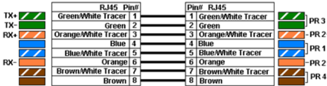
Color Standard EIA/TIA T568A Ethernet Patch Cable
