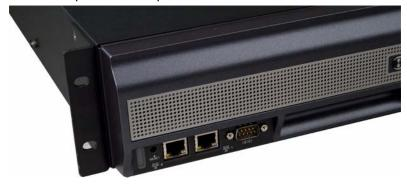
NOTE If your computer does not have a serial port, use a USB-to-serial adapter to connect the serial cable to a USB port on your computer. The USB port on the back is reserved for future use.
