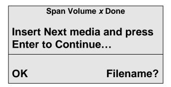
Either select OK to continue on the same form of Media. Example, if you originally spanning onto a JAZ Drive and wish to restore a 3.0 Gigabyte drive from just JAZ disks, just hit enter to continue in JAZ disks.
