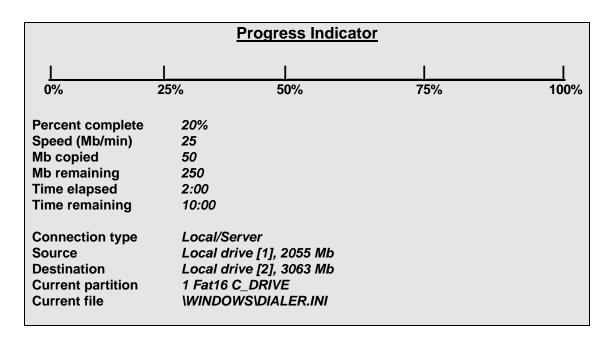
When the disk copy is complete, the target PC will need to be rebooted (as after a change made by FDISK). By default GHOST prompts with:
