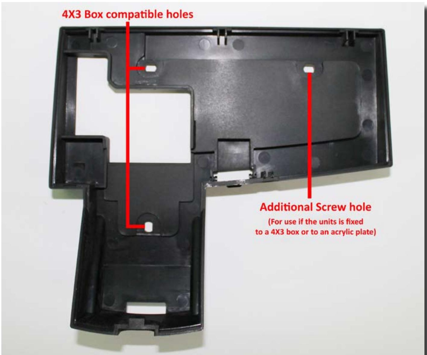
Fig. 18 – Mounting screws locations at the GAM 110 rear section. The unit can be attached to a 4X3 conduit box with 6mm screws/ 6mm sockets. For the acrylic plate unit mounting, use 4mm screws.
