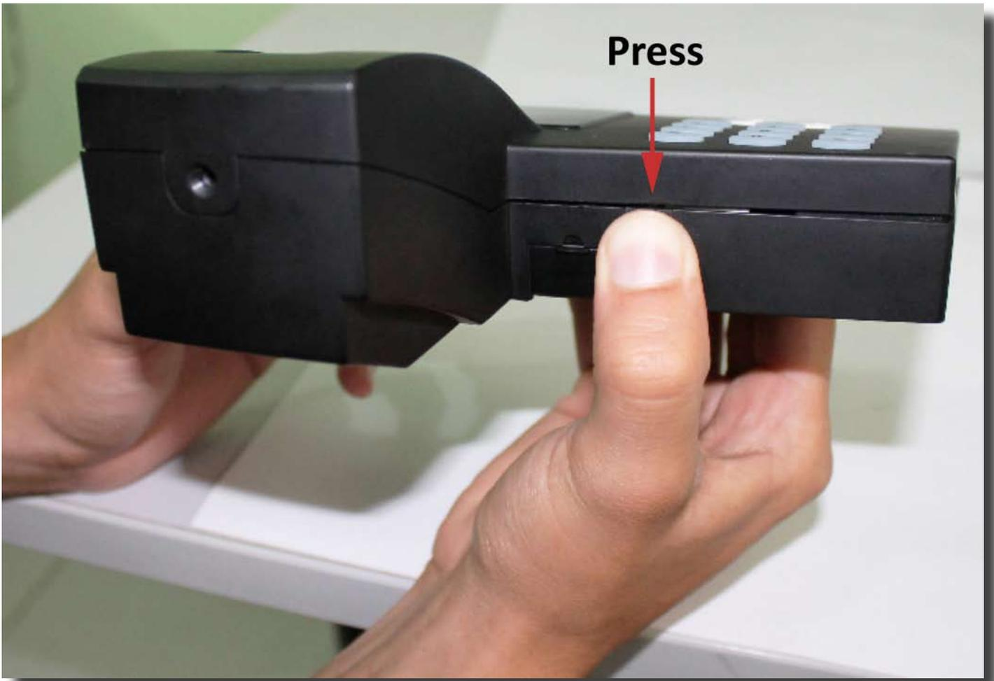
Fig.10 – Remove the screw at the bottom of the GAM 110 then use the thumb to press the enclosure as shown in the figure.
