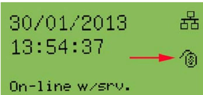
Fig 24 – GAM 110/Dual Capture Module connection confirmation icon displayed in the GAM 110 screen.
