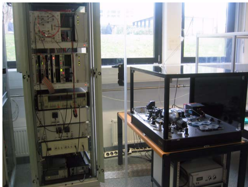
Figure 23 Light source system (laser stabilization, heterodyne assembly, control electronics) as implemented in the FTK test bed
